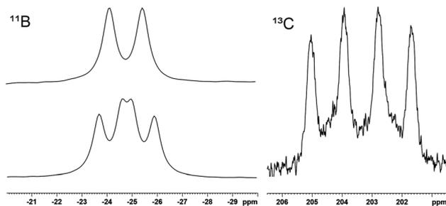
Fig. 1  $^{11}\text{B}$  NMR (128.37 MHz) (top left, natural abundance  $6$ :  $d\ ^1J_{^{31}\text{P}-^{11}\text{B}} = 168$  Hz; bottom left,  $^{13}\text{CO}$  labelled sample of  $6$ :  $dd$ ,  $^1J_{^{31}\text{P}-^{11}\text{B}} = 160.1$  Hz,  $^1J_{^{13}\text{C}-^{11}\text{B}} = 119.3$  Hz) and  $^{13}\text{C}$  NMR (100.62 MHz) carbonyl region (right) of cation  $6$ ,  $^{13}\text{CO}$  labelled ( $^1J_{^{11}\text{B}-^{13}\text{C}} = 111.6$  Hz).
