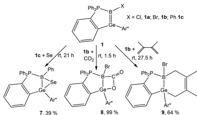
Scheme 3 Reactions of germaborene **1b** (X = Br)<sup>18</sup> and **1c** (X = Ph)<sup>65</sup> with selenium, carbon dioxide and dimethylbutadiene (Ar\* = 2,6-Trip<sub>2</sub>C<sub>6</sub>H<sub>3</sub>, Trip = 2,4,6-triisopropylphenyl).
