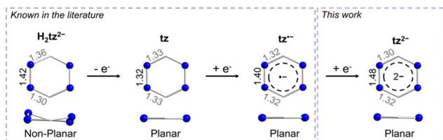
Fig. 2 Comparison of the metric parameters of the different tetrazine species. The metric parameters for the doubly deprotonated dihydrotetrazine have been extracted from  $[(\text{Cp}_2\text{Ti}(\mu\text{-H}_2\text{tz}^{2-}))_4]$ ,<sup>81</sup> while the metric parameters for the neutral tz have been extracted from  $[\text{Ag}(\text{tz})(\text{NO}_3)]_n$ .<sup>36</sup>
