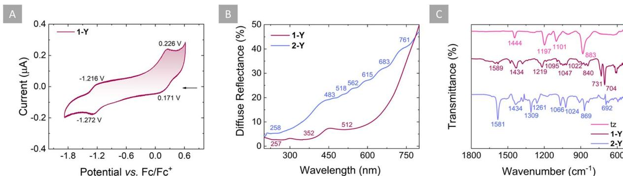
Fig. 3 (A) Cyclic voltammogram of **1-Y** measured in DCM at room temperature with  $[\text{Bu}_4\text{N}][\text{PF}_6]$  (0.1 M) as the supporting electrolyte, using a scan rate of  $0.1$   $\text{V s}^{-1}$ . (B) Diffuse reflectance spectra for **1-Y** (purple line) and **2-Y** (violet line) collected in the 200–800 nm range. (C) Zoomed-in area of the IR spectra of tz (pink), **1-Y** (purple) and **2-Y** (violet), with the respective wavenumbers. The full spectra are given in Fig. S5.†
