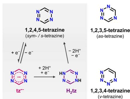
**Scheme 1** Left: Reduction pathway of *s*-tetrazine (tz) to dihydrotetrazine (H<sub>2</sub>tz) via a radical anion. The H<sub>2</sub>tz can be oxidized back to tz. Right: the structures of *as*- and *v*-tetrazine.
