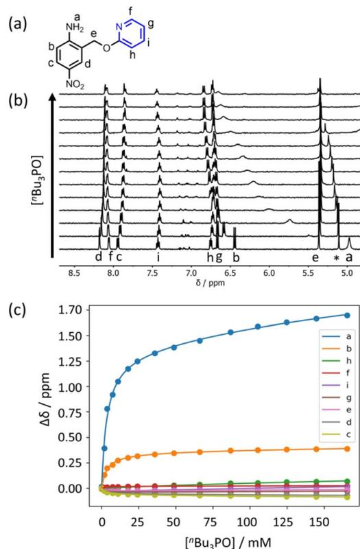
Fig. 7 (a) Proton labelling scheme for compound 4. (b) Partial 400 MHz  $^1\text{H}$  NMR spectra for titration of tri-*n*-butyl phosphine oxide into 4 (0.31 mM in *n*-octane, at 298 K). An impurity in the solvent is labelled with an asterisk. (c) The lines show the best fit of the chemical shift data (points) to a 1:2 binding isotherm ( $K_1 = 300 \text{ M}^{-1}$ ,  $K_2 = 3 \text{ M}^{-1}$ ).
