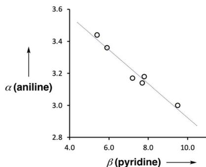
Fig. 9 Relationship between the H-bond donor parameters of compounds 2–7,  $\alpha$ (aniline), and the H-bond acceptor properties of the corresponding 4-*X*-pyridines,  $\beta$ (pyridine). The best fit line is  $y = -0.10x + 3.97$  ( $R^2 = 0.96$ ).
