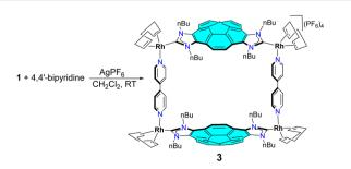
Scheme 2 Synthesis of corannulene-based metallobox 3.
