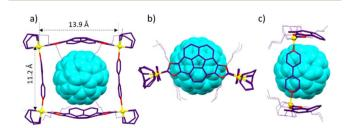
Fig. 3 (a)–(c) Show three perspectives of the molecular structure of  $C_{60}@3$ , obtained from single crystal X-ray diffraction studies. Hydrogen atoms, omitted from the figure for clarity. Counter anions (PF $_6$ ) and solvent molecules (acetone), are also omitted. Carbon atoms are in blue, nitrogen atoms in red and rhodium atoms in yellow.
