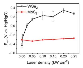
Fig. 5 Influence of laser density on onset potential  $(E_{\rm on})$  of Cu deposition on two different nanosheets.
