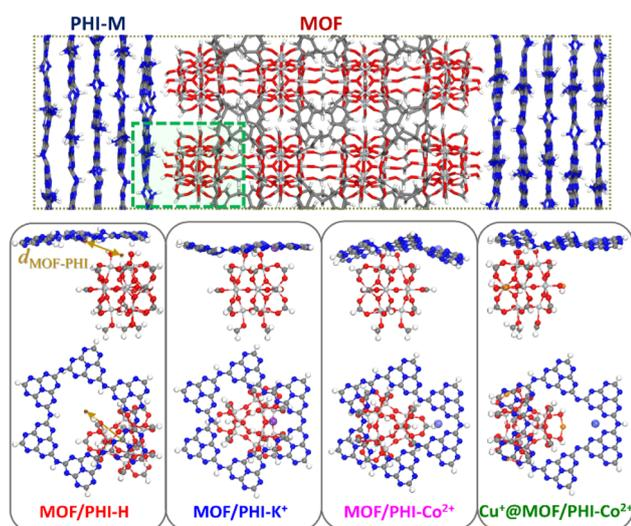
Fig. 3 Schematic illustration of the heterojunction cluster model cleaved from the force field-based MOF/PHI-M composite heterojunction (top); and lateral and top views of the DFT-optimized MOF/PHI-M heterojunction cluster models (bottom panel).
