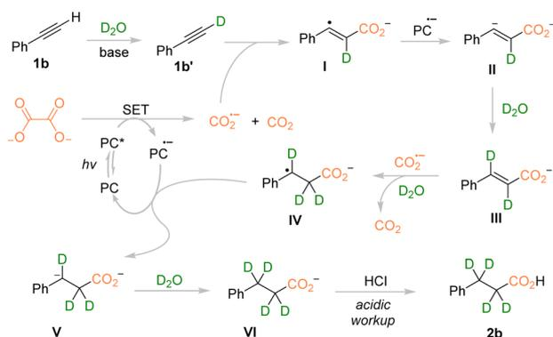
Scheme 4 Proposed mechanism for deuterocarboxylation of alkyne **1b**.
