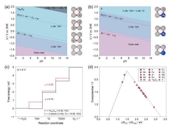
Fig. 4 Surface Pourbaix diagrams of pristine (a) and Ir-doped (b)  $Ta_2O_5$  (100) surface; free energy diagrams of the OER on the most stable surface states of pristine and Ir-doped  $Ta_2O_5$  (100) surface at pH = 0 and U = 0 V (c); OER activity trend of M-doped  $Ta_2O_5$  (100) at the most stable surface states determined by surface Pourbaix diagram analysis (d).
