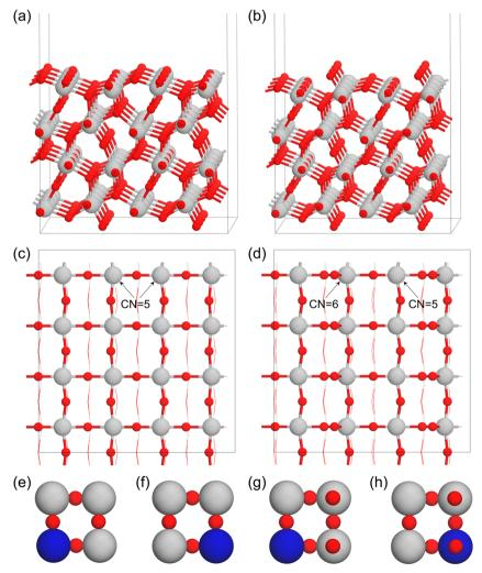
Fig. 1 The side (a and b) and top (c and d) views of Ta- and O-terminations of  $Ta_2O_5$ , as well as the metal-doped Ta-termination (e and f) and O-termination (g and h) of  $Ta_2O_5$ . (The red, grey, and bright blue spheres represent O, Ta, and dopant atoms, respectively).
