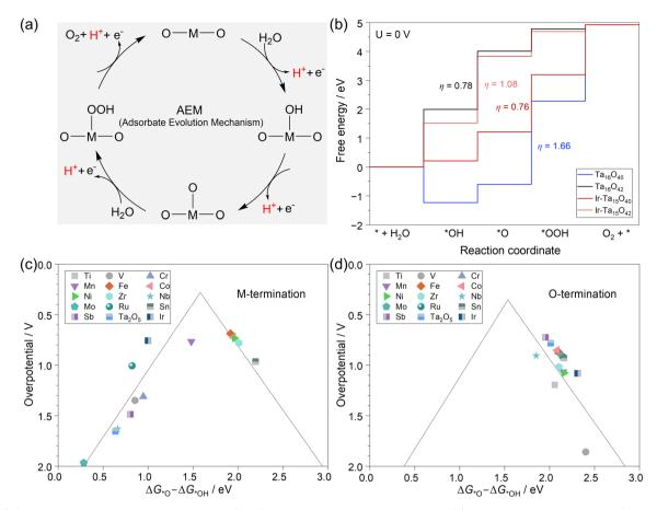
Fig. 3 (a) Classical adsorbate evolution mechanism (AEM) for the oxygen evolution reaction; (b) free energy diagrams of the OER on the two pristine and Ir-doped terminations of the  $Ta_2O_5$  (100) surface; theoretically predicted activity trends toward the OER on metal-doped (c) Ta termination (M $-Ta_{15}O_{40}$ ) and (d) O termination (M $-Ta_{15}O_{42}$ ) of the  $Ta_2O_5$  (100) surface.
