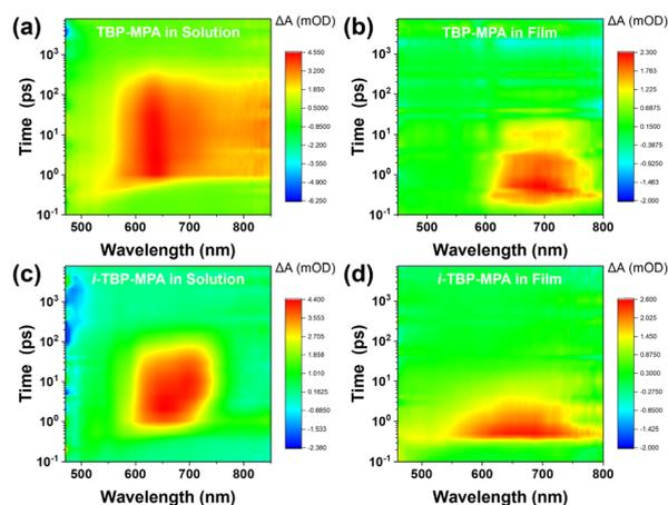
Fig. 4 Three-dimensional fs-TA spectra of (a and b) **TBP-MPA** and (c and d) *i*-**TBP-MPA** in solution (a and c) and as films (b and d).
