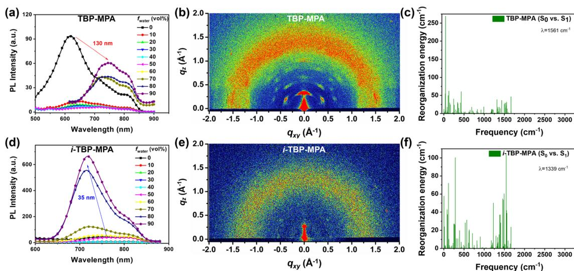
Fig. 3 PL spectra of (a) **TBP-MPA** and (d) *i*-**TBP-MPA** in a THF/H<sub>2</sub>O mixture with different  $f_{\text{water}}$ . 2D GIWAXS patterns of (b) **TBP-MPA** and (e) *i*-**TBP-MPA** films. Calculated reorganization energy (environment: toluene) of (c) **TBP-MPA** and (f) *i*-**TBP-MPA** at different wavenumbers.
