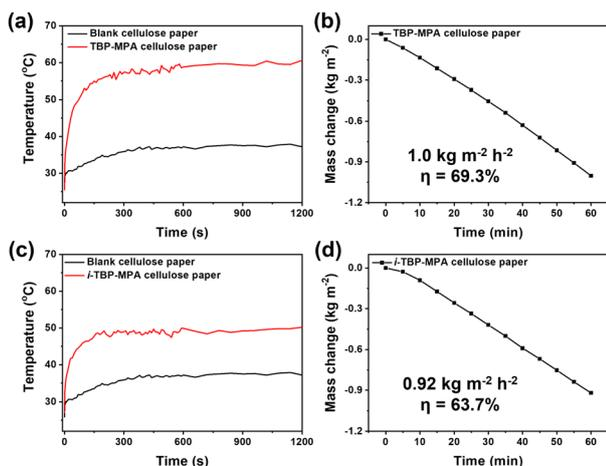
Fig. 5 Temperature change curves of (a) TBP-MPA cellulose paper and (c) *i*-TBP-MPA cellulose paper and blank cellulose papers under a power density of 1 kW m<sup>-2</sup> upon 20 min irradiation. Water evaporation curves of (b) TBP-MPA cellulose paper and (d) *i*-TBP-MPA cellulose paper.
