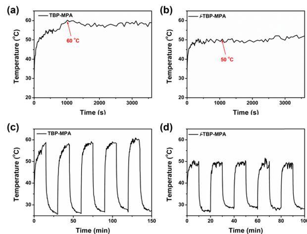
Fig. 2 Temperature change curves of (a) TBP-MPA and (b) *i*-TBP-MPA powders under 1 sun irradiation for 1 h. Photobleaching resistance properties during five cycles of on-off processes of (c) TBP-MPA and (d) *i*-TBP-MPA powders.
