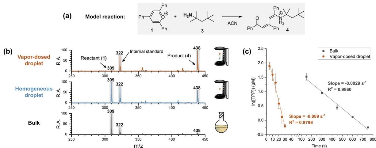
Fig. 2 Reaction acceleration in vapor-dosed droplet. (a) Model reaction. (b) Comparison of vapor-dosed droplet (top panel), individual homogeneous droplet (middle panel), and bulk (bottom panel). The reaction time was 30 s. (c) Kinetics plots for vapor-dosed droplet and bulk at room temperature (note dramatically different time scales).
