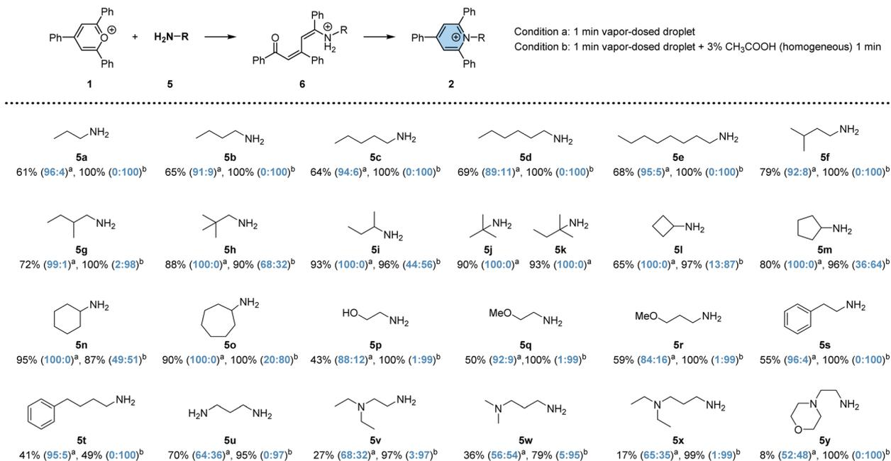
**Scheme 1** Substrate scope of Katritzky reactions in vapor-dosed droplets. The overall yield of intermediate **6** and final product **2** was obtained by performing the reactions under conditions a or b. The ratio between product **6** and **2** is shown in brackets, annotated in blue. A three-microliter (3  $\mu$ L) droplet was used in each case, yielding the product on a microgram scale.
