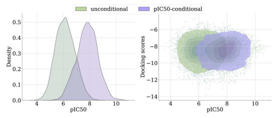
Fig. 8 Left: density plot comparing unconditional with  $pIC_{50}$ -conditional sampling. Right: scatter heatmap overlap of unconditional and  $pIC_{50}$ -conditional samples comparing docking scores and (predicted)  $pIC_{50}$  values.
