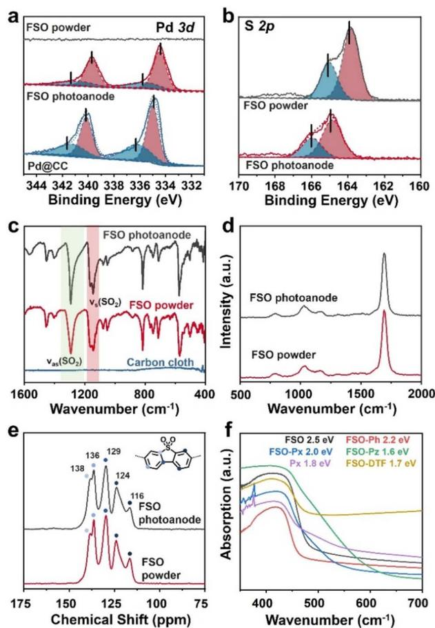
Fig. 3 (a) Pd 3d and (b) S 2p XPS spectra of FSO. (c) FTIR spectra, (d) Raman spectra, and (e) <sup>13</sup>C CP/MAS NMR chemical shift of FSO. (f) UV/vis DRS of the linear polymer based photoanodes.
