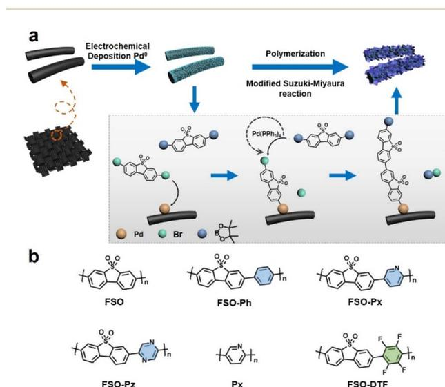
Fig. 1 (a) Proposed mechanism of the growth procedure of the linear conjugated polymer photocatalysts on carbon cloth *via* a modified Suzuki–Miyaura reaction. (b) Chemical structures of the linear semiconductor polymers used in this study.
