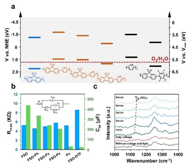
Fig. 5 (a) Bandgap of the linear semiconductor polymers. (b) The  $R_{\text{ct,ss}}$  and  $C_{\text{ss}}$  of the linear polymer based photoanode obtained from Nyquist plot of EIS (inset: the equivalent circuit for EIS). (c) Time-resolved *in situ* Raman spectra of the FSO photoanode for water oxidation reaction.
