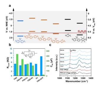
Fig. 5 (a) Bandgap of the linear semiconductor polymers. (b) The  $R_{\rm ct,ss}$  and  $C_{\rm ss}$  of the linear polymer based photoanode obtained from Nyquist plot of EIS (inset: the equivalent circuit for EIS). (c) Timeresolved *in situ* Raman spectra of the FSO photoanode for water oxidation reaction.
