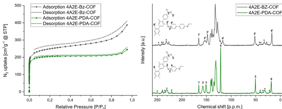
Fig. 4 Nitrogen adsorption isotherms at 77 K (left) of **4A2E-PDA-COF** (green) and **4A2E-Bz-COF** (grey).  $^{13}\text{C}$ -MAS NMR of **4A2E-PDA-COF** (grey) and **4A2E-Bz-COF** (green). Asterisks indicate spinning side bands.
