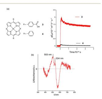
Fig. 5 (a) FP-TRMC profiles for as-synthesized 3-HOF (red) and 4 (black). (b) Transient absorption spectrum of 3-HOF in a PMMA film recorded at 0-10 ms after pulse excitation at 355 nm (6.4  $\times$  10<sup>15</sup> photons per cm<sup>2</sup>).
