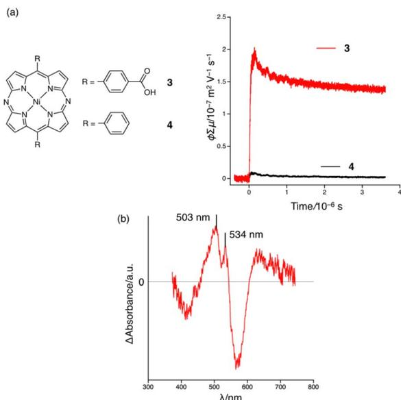
Fig. 5 (a) FP-TRMC profiles for as-synthesized **3-HOF** (red) and **4** (black). (b) Transient absorption spectrum of **3-HOF** in a PMMA film recorded at 0–10 ms after pulse excitation at 355 nm ( $6.4 \times 10^{15}$  photons per  $\text{cm}^2$ ).
