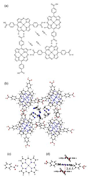
Fig. 2 (a) Schematic illustration of the crystal structure of 3-HOF. (b) Top view of the X-ray crystal structure of 3-HOF. (c) Double hydrogenbonding interactions between the diazaporphyrin cores and the carboxyphenyl groups. (d) Packing structure of three stacked molecules of 3.
