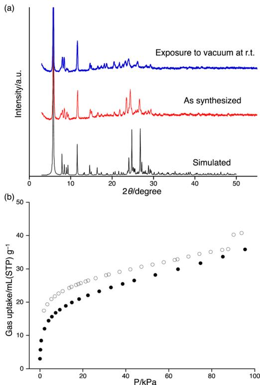
Fig. 3 (a) PXRD patterns of the as-synthesized sample (red) and the sample exposed to vacuum at r.t. (blue), together with the simulated PXRD pattern (black) of **3-HOF**. (b) Adsorption (●)/desorption (○) isotherms for CO<sub>2</sub> at 195 K.
