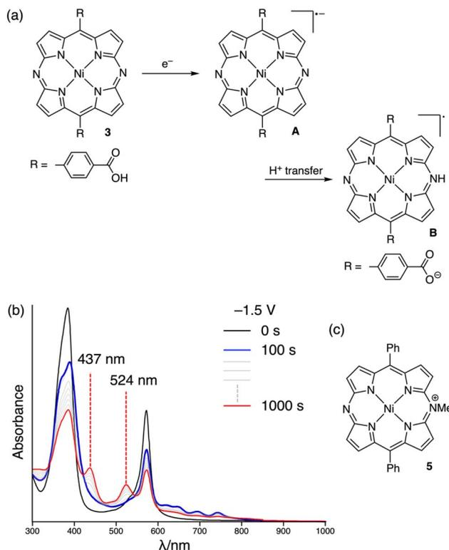
Fig. 4 (a) Schematic illustration of the one-electron reduction of **3** involving proton transfer. (b) Change in the absorption spectrum of **3** in DMF upon one-electron reduction. (c) Structure of *N*-methyl-diazaporphyrinium cation **5**.
