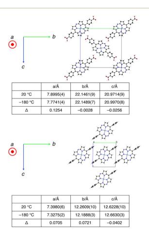
Fig. 7 Crystal structures and dimensions of the crystal lattice at different temperatures for 3-HOF (top) and 4 (bottom).
