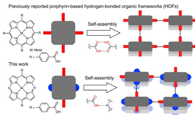
Fig. 1 Schematic representation of porphyrin-(previous work; top) and diazaporphyrin-based HOFs (this work; bottom).
