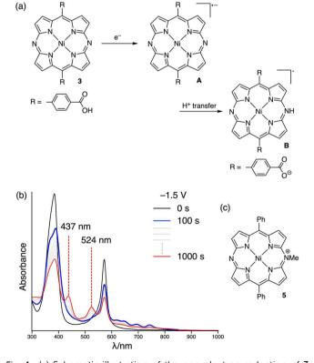
Fig. 4 (a) Schematic illustration of the one-electron reduction of 3 involving proton transfer. (b) Change in the absorption spectrum of 3 in DMF upon one-electron reduction. (c) Structure of N-methyl-diazaporphyrinium cation 5.
