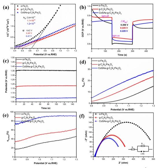
Fig. 6 (a) M–S plots; (b) OCP transient decay curves; (c) potential ( $V_{RHE}$ ) versus time for the photoelectrodes at 1 mA cm<sup>-2</sup>; (d)  $\eta_{bulk}$ ; (e)  $\eta_{surface}$ ; (f) EIS of  $\alpha$ -Fe<sub>2</sub>O<sub>3</sub>, g-C<sub>3</sub>N<sub>4</sub>/Fe<sub>2</sub>O<sub>3</sub>, CoSAs-g-C<sub>3</sub>N<sub>4</sub>/Fe<sub>2</sub>O<sub>3</sub> photoanodes.
