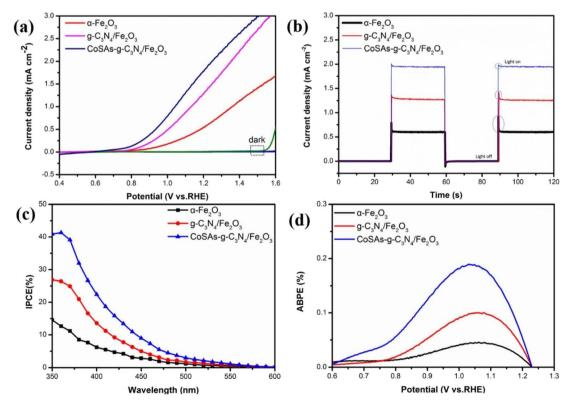
Fig. 5 (a) LSV curves; (b) transient photocurrent measurements at 1.23  $V_{RHE}$ ; (c) IPCE curves; (d) ABPE curves of  $\alpha$ -Fe<sub>2</sub>O<sub>3</sub>, g-C<sub>3</sub>N<sub>4</sub>/Fe<sub>2</sub>O<sub>3</sub>, and CoSAs-g-C<sub>3</sub>N<sub>4</sub>/Fe<sub>2</sub>O<sub>3</sub> photoanodes.
