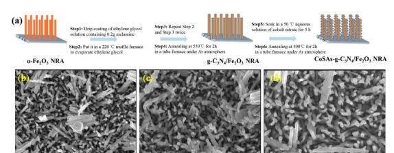
Fig. 1 (a) Schematic of the CoSAs-g-C $_3$ N $_4$ /Fe $_2$ O $_3$  NRA photoanode preparation process. Top-view SEM images of (b)  $\alpha$ -Fe $_2$ O $_3$ ; (c) g-C $_3$ N $_4$ /Fe $_2$ O $_3$ ; (d) CoSAs-g-C $_3$ N $_4$ /Fe $_2$ O $_3$ .
