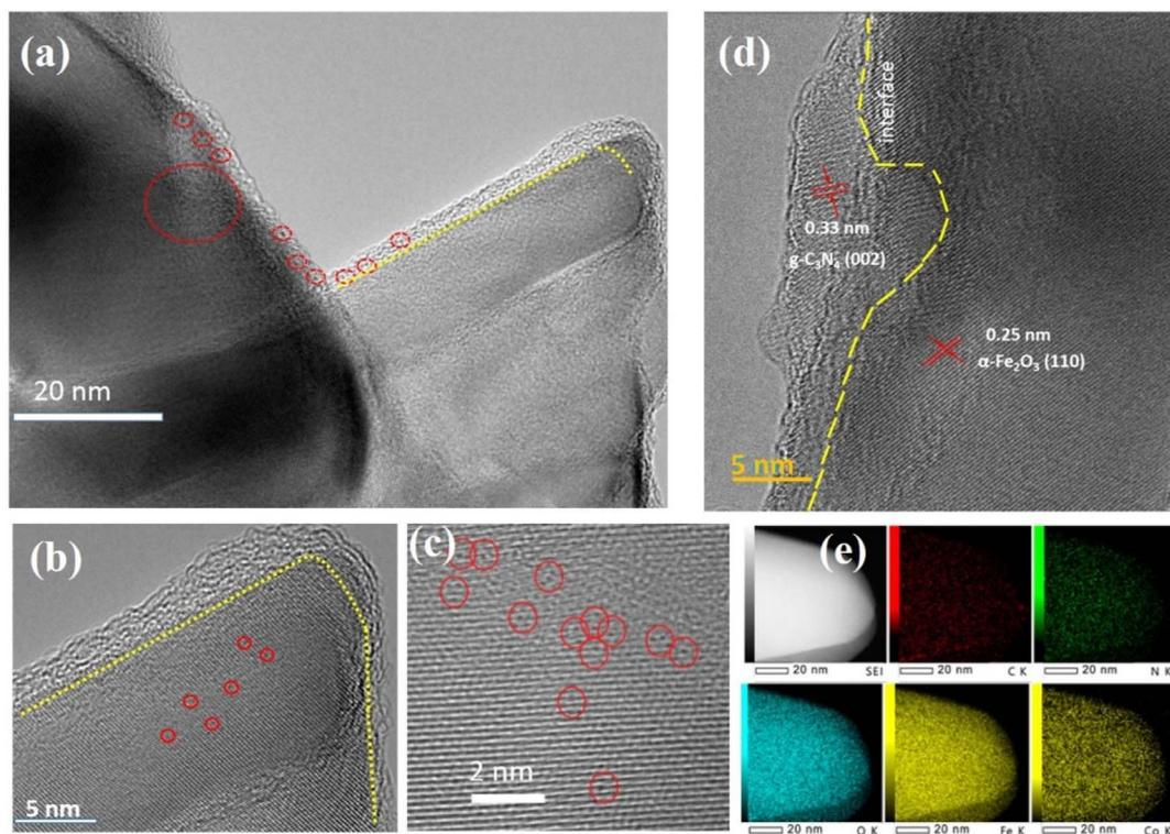
Fig. 2 (a)–(c) Atomic-resolution TEM images of CoSAs-g-C<sub>3</sub>N<sub>4</sub>/Fe<sub>2</sub>O<sub>3</sub> NR (CoSAs are highlighted by red circles); (d) and (e) HRTEM image and EDS mapping of Co, Fe, O, C, and N for CoSAs-g-C<sub>3</sub>N<sub>4</sub>/Fe<sub>2</sub>O<sub>3</sub> NR.
