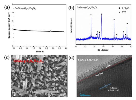
Fig. 7 (a) Photocurrent density stability of CoSAs-g- $C_3N_4$ /Fe $_2O_3$  photoanodes at 1.23  $V_{RHE}$ ; (b) XRD pattern; (c) SEM; (d) HRTEM of CoSAs-g- $C_3N_4$ /Fe $_2O_3$  photoanodes after long-term stability tests.
