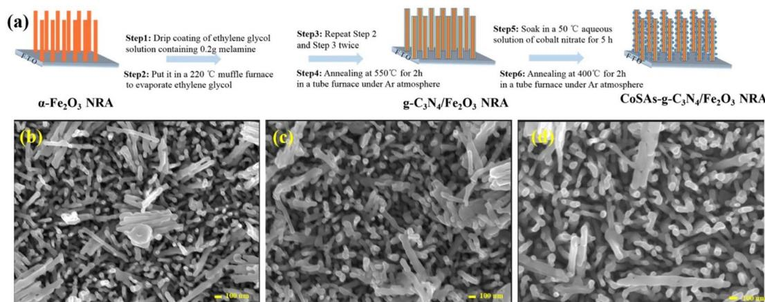
Fig. 1 (a) Schematic of the CoSAs-g-C<sub>3</sub>N<sub>4</sub>/Fe<sub>2</sub>O<sub>3</sub> NRA photoanode preparation process. Top-view SEM images of (b)  $\alpha$ -Fe<sub>2</sub>O<sub>3</sub>; (c) g-C<sub>3</sub>N<sub>4</sub>/Fe<sub>2</sub>O<sub>3</sub>; (d) CoSAs-g-C<sub>3</sub>N<sub>4</sub>/Fe<sub>2</sub>O<sub>3</sub>.
