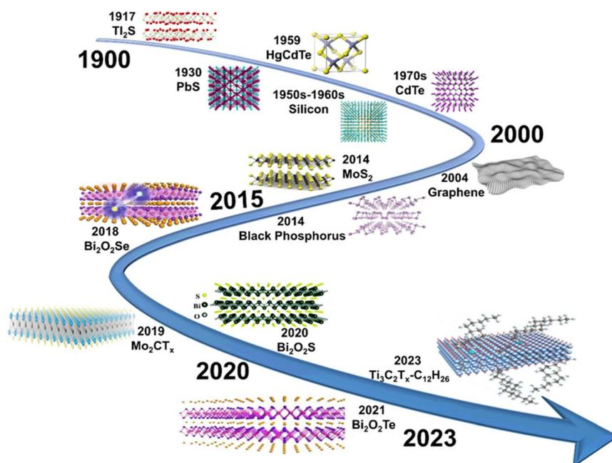
Fig. 2 Timelines of the compounds developed for infrared photodetectors.
