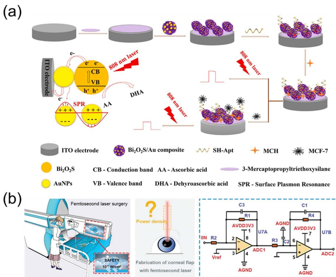
Fig. 11 (a) The fabrication of the PEC aptamer sensor and the detection mechanism of tumor cells.<sup>182</sup> (b)  $\text{Ti}_3\text{C}_2\text{T}_x$ -RAN photodetector monitors laser density display and laser density monitoring system circuit diagram during femtosecond laser surgery.<sup>183</sup>
