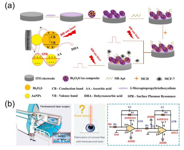
Fig. 11 (a) The fabrication of the PEC aptamer sensor and the detection mechanism of tumor cells.  $^{182}$  (b)  $T_{13}C_2T_x$ -RAN photodetector monitors laser density display and laser density monitoring system circuit diagram during femtosecond laser surgery.  $^{183}$
