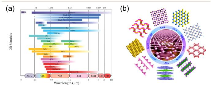
Fig. 5 (a) Comparison of the response wavelength ranges of different 2D materials.<sup>41</sup> (b) Diagram of the crystal structures of the well-known 2D compounds.<sup>71</sup>
