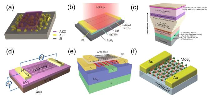
Fig. 4 (a) Schematic diagram of the broad-band NIR Si Schottky photodetector.<sup>55</sup> (b) Schematic illustration of the B-doped Si-QD/MCT device structure.<sup>56</sup> (c) Structure diagram of the photodetector based on the InGaAs material.<sup>57</sup> (d) Schematic diagram of the graphene-based photodetector.<sup>13</sup> (e) Schematic diagram of the black phosphorus infrared photodetector.<sup>14</sup> (f) Schematic diagram of the MoS<sub>2</sub> infrared photodetector.<sup>58</sup>
