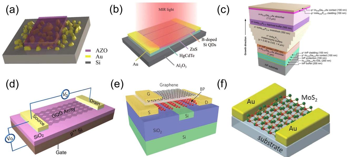
Fig. 4 (a) Schematic diagram of the broad-band NIR Si Schottky photodetector.<sup>55</sup> (b) Schematic illustration of the B-doped Si-QD/MCT device structure.<sup>56</sup> (c) Structure diagram of the photodetector based on the InGaAs material.<sup>57</sup> (d) Schematic diagram of the graphene-based photodetector.<sup>13</sup> (e) Schematic diagram of the black phosphorus infrared photodetector.<sup>14</sup> (f) Schematic diagram of the MoS<sub>2</sub> infrared photodetector.<sup>58</sup>
