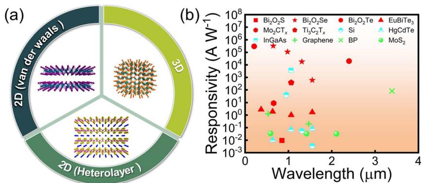
Fig. 6 (a) Comparison of the crystal structures of typical 2D, heterolayered, and 3D compounds. (b) The reported responsivities of photodetectors of typical 2D, heterolayered, and 3D compounds in the UV to MIR region.
