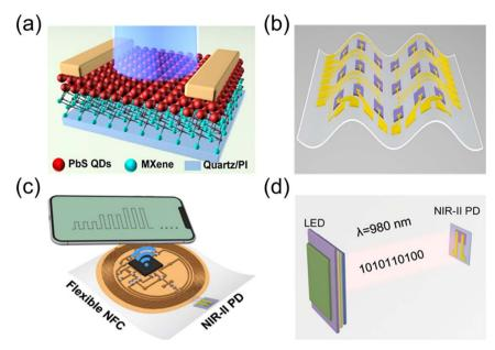
Fig. 12 (a) MXene/PbS infrared photodetector schematic diagram.<sup>185</sup> (b) A skin-like bilayer photodetector array was prepared on the PI substrate.<sup>185</sup> (c) A schematic diagram of a wireless photodetection system using flexible NFC and NIR-II photodetectors.<sup>185</sup> (d) The schematic diagram of optical communication through NIR-II light.<sup>185</sup>
