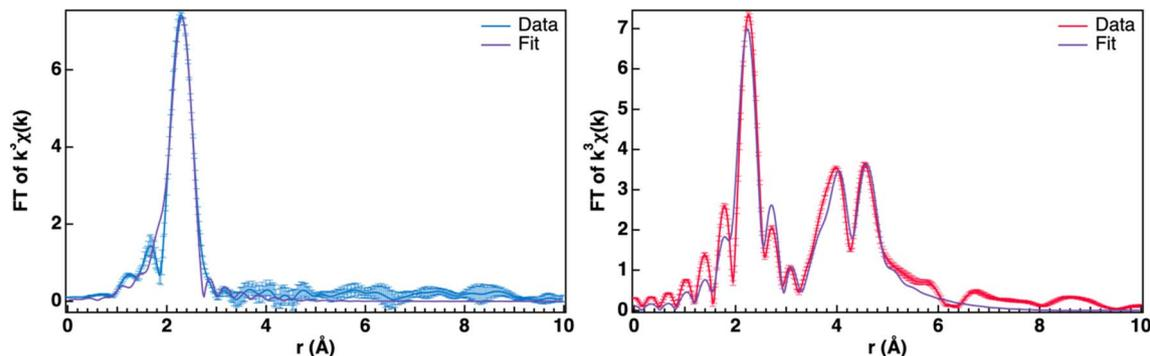
Fig. 6 EXAFS U  $L_3$ -edge spectra of 1-US<sub>2</sub> (blue, left) and 2-US<sub>2</sub> (pink, right) samples, including fits (purple) and error bars.
