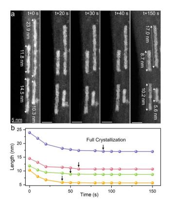
Fig. 2 In situ STEM observation of the growth process of  $U_4O_9$  nanorods in SWCNTs stimulated by an e-beam. (a) Time-sequential HAADF-STEM images of  $U_4O_9$  formed at different stages. (b) The length of  $U_4O_9$  nanorods versus irradiation time derived from analysis of STEM images. The full crystallization time for each  $U_4O_9$  nanorod is marked by arrows.
