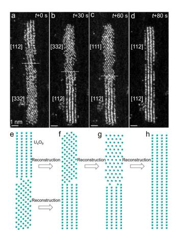
Fig. 5 Structural reconstruction-assisted growth of single-crystal  $U_4O_9$  nanorod within an SWCNT. (a–d) Time-sequential HAADF-STEM images. (e–h) Corresponding atomic models of  $U_4O_9$  reconstruction processes derived from STEM images. The O atoms are invisible.
