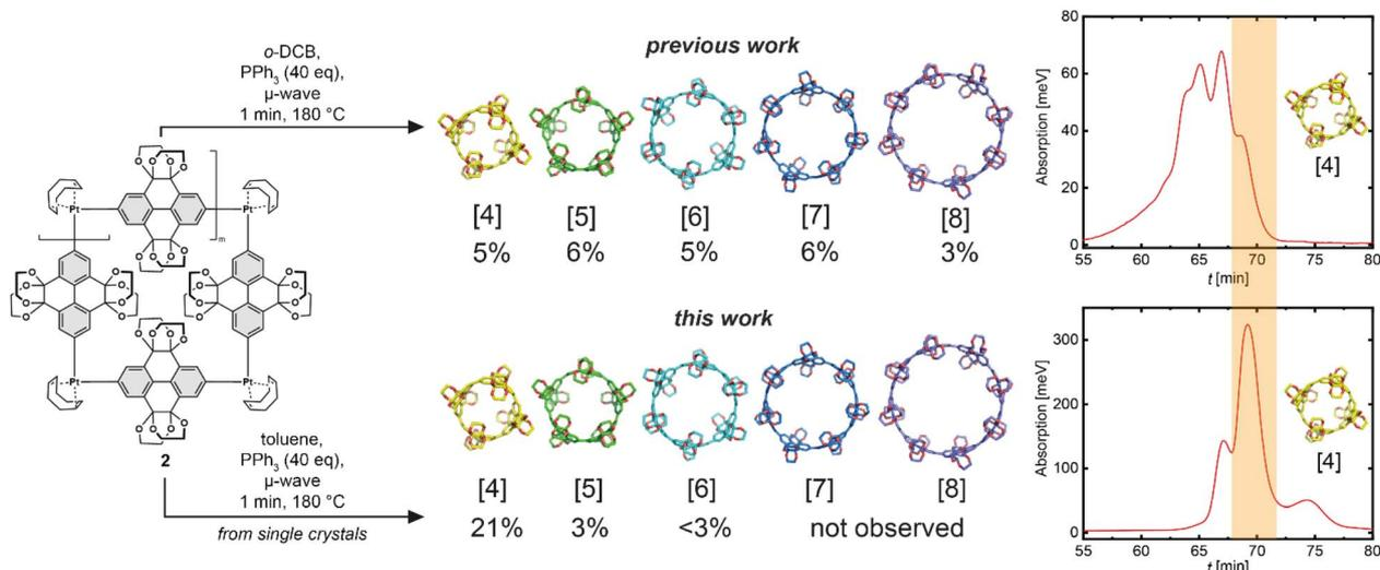
Fig. 3 Comparison of the reductive elimination from a sample containing different ring sizes of the platinum metallacycle (previous work) and a sample of single-crystals of the four membered metallacycle (this work), with corresponding yields and the rGPC chromatograms of the crude reaction mixture.
