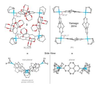
Fig. 2 Single-crystal X-ray structure of platinum macrocycle 2 with side view and Yamago and co-workers' 2014 platinum macrocycle<sup>44</sup> for comparison. Ellipsoids are shown at 50% probability; hydrogen atoms and solvent molecules are omitted for clarity. Colour code: carbon, grey; oxygen, red.
