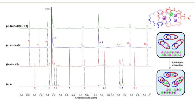
Fig. 5 Solid—liquid extraction studies of alkali metal bromide salts, showing truncated <sup>1</sup>H NMR spectra of: (a) free catenane receptor 4, and post-extraction spectra of 4 following treatment with (b) 10 mg KBr; (c) 10 mg NaBr; (d) 5 mg NaBr and 5 mg KBr (CDCl<sub>3</sub>, 298 K, 500 MHz). The inset on the right shows the structure of 4 bound to an MX ion-pair (top) and a schematic illustrating the SLE experiment (bottom).
