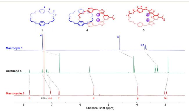
Fig. 2 Stacked <sup>1</sup>H NMR spectra of macrocycle 1 (top), [2]catenane 4 (middle) and XB macrocycle 5 (bottom) (500 MHz, CDCl<sub>3</sub>, 298 K).
