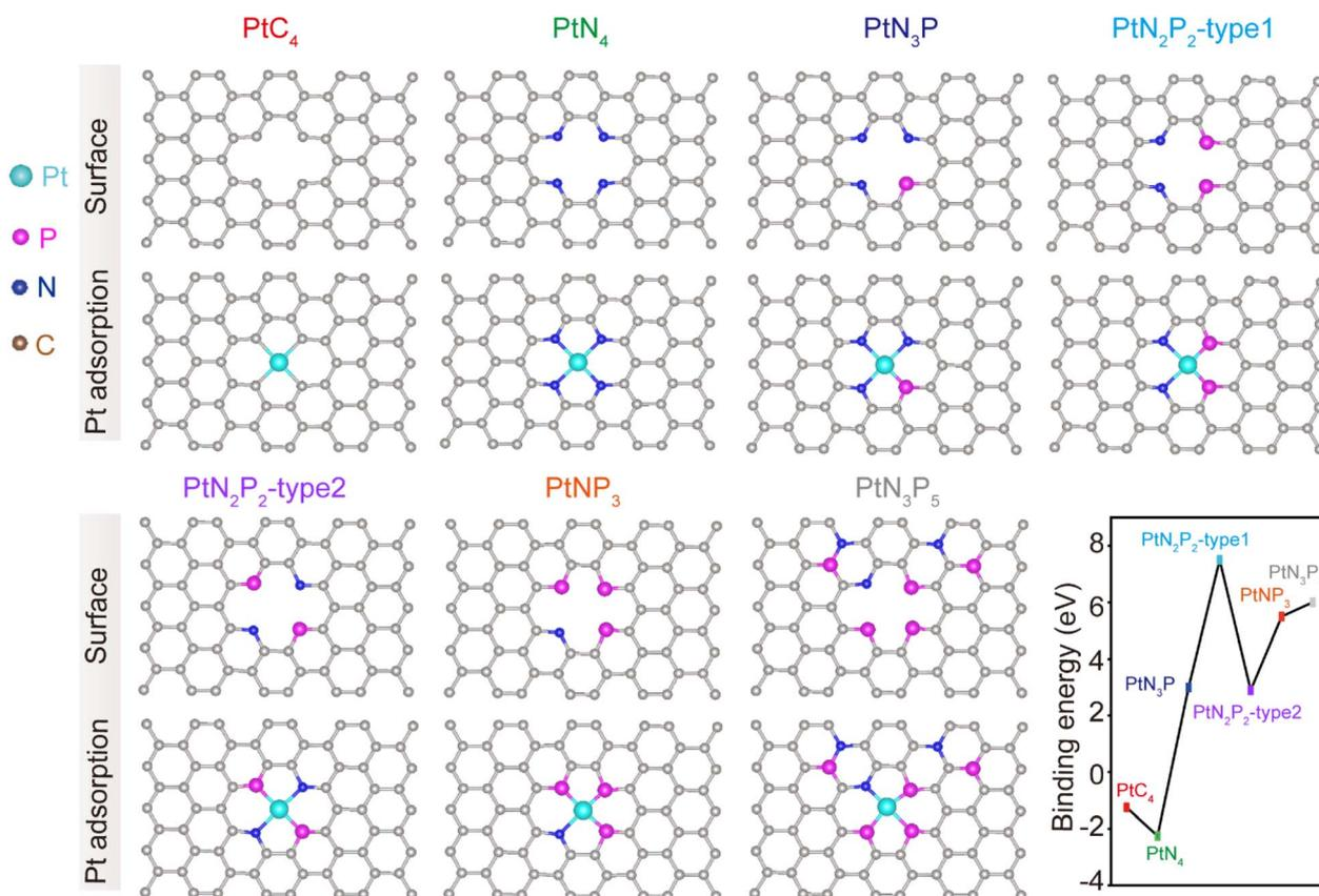
Fig. 1 Prediction of the structural stability of Pt single atoms with different first coordination environment and calculated binding energy of Pt atom anchored on the doped-graphene ( $PtC_4$ ,  $PtN_4$ ,  $PtN_3P$ ,  $PtN_2P_2$ -type 1,  $PtN_2P_2$ -type 2,  $PtNP_3$ ,  $PtN_3P_5$ ) monolayer. All energies are given in eV.
