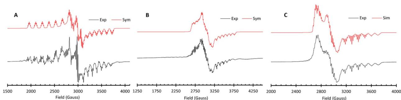
Fig. 7 (A) X-band (9.4 GHz) EPR spectrum of a 2.5 mM frozen solution of **1** in THF at 30 K at a power of 30 dB. (B) X-band (9.4 GHz) EPR spectrum of a 2.5 mM frozen solution of **2** in THF at 30 K at a power of 20 dB. (C) X-band (9.4 GHz) EPR spectrum of a saturated frozen solution of **6** in THF at 30 K at a power of 30 dB.
