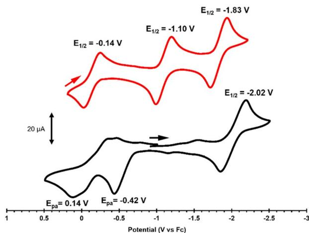
Fig. 3 Cyclic voltammograms of **1** (bottom, black) and **2** (top, red) in 0.1 M [ $n\text{-Bu}_4\text{N}$ ][PF $_6$ ] solution (scan rate = 100 mV s $^{-1}$ ). All potentials are referenced to Fc/Fc $^+$ .
