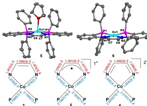
Fig. 5 (Top) Displacement ellipsoid (50%) representations of 5 (Left) and 6 (Right). All H atoms, solvate molecules, and PF<sub>6</sub><sup>−</sup> anions were omitted for clarity. (Bottom) Comparison of the metal–ligand and N–C–C–N bond metrics of 2, 5, and 6.
