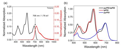
Fig. 2 (a) Absorption and emission spectra of pyrPDI-tpPDI in toluene. (b) Absorption of pyrPDI, tpPDI, and pyrPDI-tpPDI in toluene normalized to their corresponding peak maxima.
