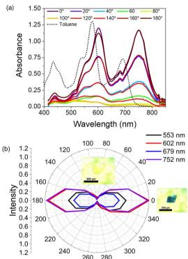
**Fig. 3** Absorption spectra of a **pyrPDI-tpPDI** single crystal. (a) Polarization resolved steady-state absorption spectrum of a **pyrPDI-tpPDI** single crystal. (b) Radial absorption plot of four wavelengths with micrographs at 0 and 90° polarization.
