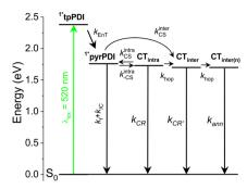
Fig. 6 Jablonski diagram of pyrPDI-tpPDI single crystal at room temperature and the rate constants for energy transfer (EnT), intermolecular charge transfer (CS, inter), intramolecular charge transfer (CS, intra), charge hopping (hop), and CT annihilation (ann).
