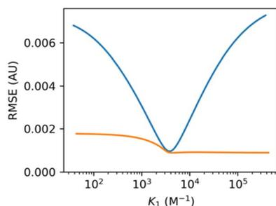
Fig. 2 Relationship between the RMSE and the value of  $K_1$  for the UV/vis titration data in Fig. 1 fitted using a model allowing for absorption of the host, free guest, and 1:1 complex (blue) or a model allowing for absorption of the host, free guest, 1:1 complex and 1:2 complex (orange).
