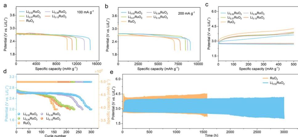
Fig. 4 Discharge profiles of Li–O<sub>2</sub> batteries with RuO<sub>2</sub> or Li<sub>x</sub>RuO<sub>2</sub> cathode at a current density of (a) 100 mA g<sup>-1</sup> and (b) 200 mA g<sup>-1</sup>. The first-cycle charge–discharge curve (c), terminal discharge voltages and corresponding capacity (d) and cycling stability (e) of Li–O<sub>2</sub> batteries with RuO<sub>2</sub> or Li<sub>x</sub>RuO<sub>2</sub> cathode at 100 mA g<sup>-1</sup> with a limited capacity of 500 mA h g<sup>-1</sup>.
