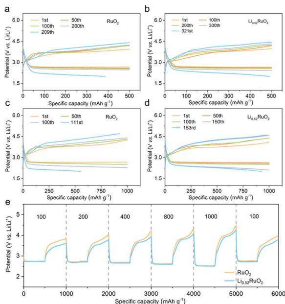
Fig. 5 Cycling performance of RuO<sub>2</sub> and Li<sub>x</sub>RuO<sub>2</sub> in Li–O<sub>2</sub> batteries with a cutoff capacity of (a and b) 500 mA h g<sup>-1</sup> or (c and d) 1000 mA h g<sup>-1</sup> at a current density of 500 mA g<sup>-1</sup>. (e) Rate performance of RuO<sub>2</sub> and Li<sub>0.52</sub>RuO<sub>2</sub> under current density changing from 100 to 1000 mA g<sup>-1</sup>.
