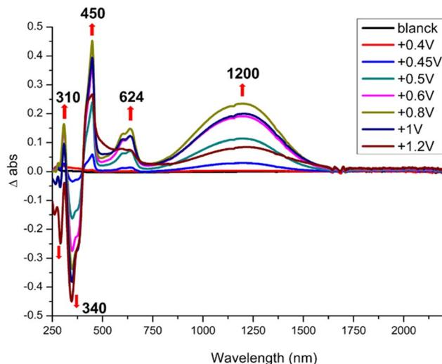
Fig. 3 Differential UV-vis-NIR absorption spectra upon incremental oxidation of **1** into **1'**, performed in CH<sub>2</sub>Cl<sub>2</sub> with 0.2 M Bu<sub>4</sub>NPF<sub>6</sub>. Potentials in V vs. SCE.
