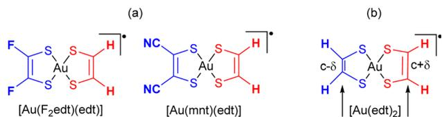
Scheme 4 Model complexes theoretically investigated with (a)  $[\text{Au}(\text{R,Redt})(\text{edt})]^*$  ( $\text{R}=\text{F}, \text{CN}$ ) complexes, (b)  $[\text{Au}(\text{edt})_2]^*$  complexes with constrained  $\text{C}=\text{C}$  bonds.
