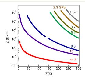
Fig. 8 Temperature and pressure dependence of the resistivity of  $1^{\prime}$  up to 11.5 GPa.
