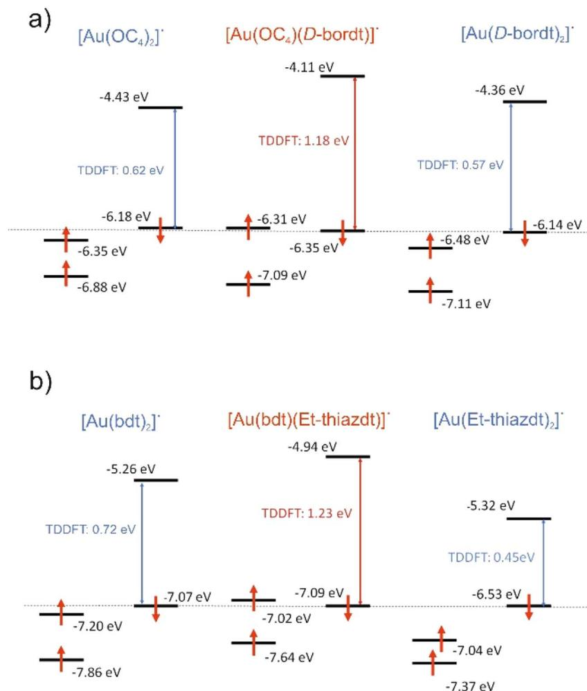
Fig. 6  $[\text{Au}(\text{OC}_4)(D\text{-bordt})]^+$  (a) and  $[\text{Au}(\text{bdt})(\text{Et-thiazdt})]^+$  (b): first significant low energy transition (SOMO-1  $\rightarrow$  LUMO), SOMO, SOMO-1 and LUMO levels as calculated by TDDFT for the asymmetric and the two associated symmetric complexes. For convenience, the energy of the  $\beta$  SOMO-1 levels have been aligned.
