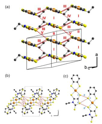
Fig. 7 (a) Layers of the crystal structure of the radical 1' where the different intermolecular interactions are noted. The S···S contacts shorter than 3.8 Å are shown as dotted red lines. (b) Top view of the layer. (c) Intermolecular interaction III: the + and - signs refer to the sign of the S  $p_z$  orbital in the SOMO showing that interactions  $\bf a$  and  $\bf a'$  almost cancel.
