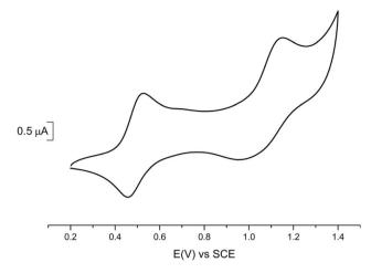
Fig. 2 Cyclic voltammetry of 1 performed in 0.1 M  $Bu_4NPF_6$  in  $CH_2Cl_2$  at 100 mV s<sup>-1</sup> scan rate.
