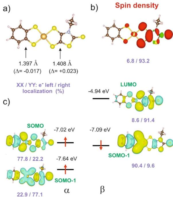
Fig. 4 [Au(bdt)(Et-thiazdt)]<sup>+</sup> complex **1'**: (a) C=C optimized bond lengths, (b) spin density, and (c) spin-orbitals around the SOMO. The pairs of violet numbers indicate the left/right distribution (%) of the spin density in (b) or the electron distribution in a given spin-orbital in (c). In (a) the values in parenthesis are the bond length changes with respect to the corresponding symmetric complexes.
