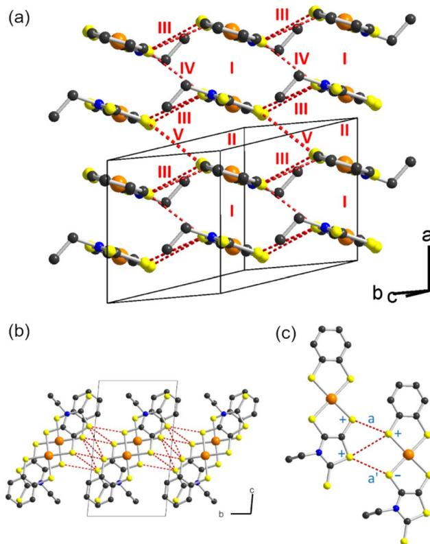
Fig. 7 (a) Layers of the crystal structure of the radical  $\mathbf{1}'$  where the different intermolecular interactions are noted. The S...S contacts shorter than 3.8 Å are shown as dotted red lines. (b) Top view of the layer. (c) Intermolecular interaction III: the + and - signs refer to the sign of the  $S_{p_z}$  orbital in the SOMO showing that interactions  $a$  and  $a'$  almost cancel.
