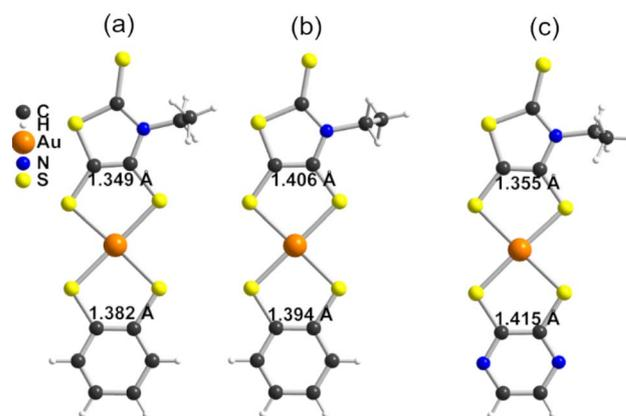
Fig. 1 Molecular structures of, (a) the anionic  $[\text{Au}(\text{bdt})(\text{Et-thiazdt})]^{-1}$  complex in **1**, (b) the neutral radical  $[\text{Au}(\text{bdt})(\text{Et-thiazdt})]^{\cdot}$  complex in **1'**, (c) the anionic  $[\text{Au}(\text{pzdt})(\text{Et-thiazdt})]^{-1}$  complex in **2** (only one of the two crystallographically independent  $[\text{Au}(\text{pzdt})(\text{Et-thiazdt})]^{-1}$  moieties is shown).
