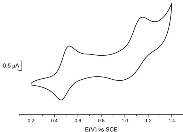
Fig. 2 Cyclic voltammetry of **1** performed in 0.1 M Bu<sub>4</sub>NPF<sub>6</sub> in CH<sub>2</sub>Cl<sub>2</sub> at 100 mV s<sup>-1</sup> scan rate.
