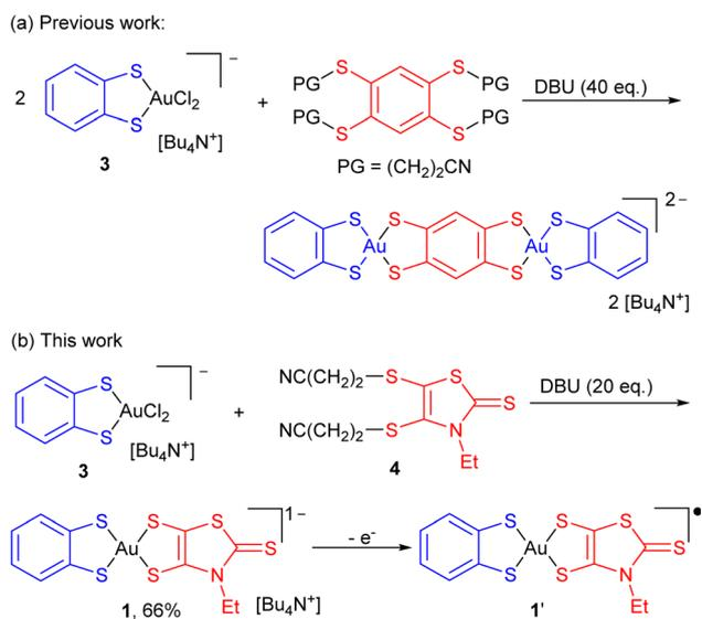
Scheme 2 Synthetic paths to mixed-ligand bis-dithiolene complexes, and preparation of  $[\text{nBu}_4\text{N}][\text{Au}(\text{bdt})(\text{Et-thiazdt})]^-$  **1**.
