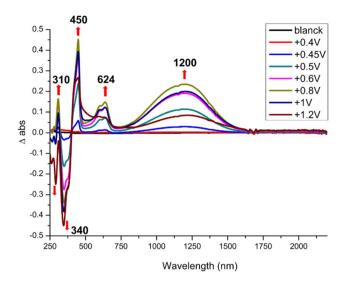
Fig. 3 Differential UV-vis-NIR absorption spectra upon incremental oxidation of  $\bf 1$  into  $\bf 1'$ , performed in CH<sub>2</sub>Cl<sub>2</sub> with 0.2 M Bu<sub>4</sub>NPF<sub>6</sub>. Potentials in V vs. SCE.
