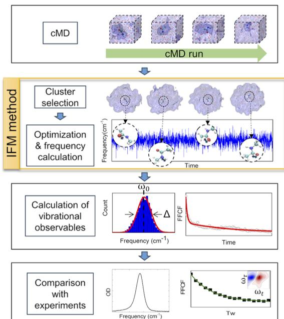
Fig. 2 Procedure followed for the development and testing of the IFM method.
