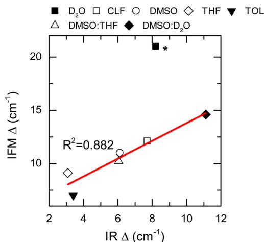
Fig. 5 Frequency fluctuation amplitudes ( $\Delta$ ) calculated by the IFM vs. determined from the IR spectra (data points). Linear fit corresponds to the red line. Star (\*) NMA in the  $\text{D}_2\text{O}$   $\Delta$  value was not included into the fit.
