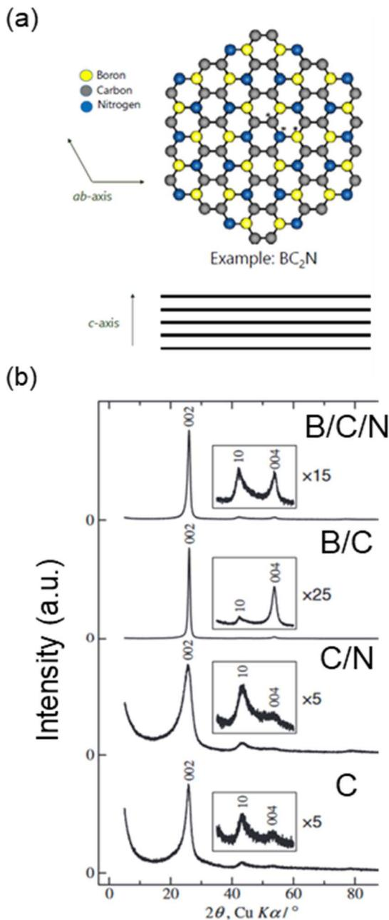
Fig. 14 Structure of B/C/N materials. (a) Graphite-like network of B/C/N (example:  $\text{BC}_2\text{N}$ ). (b) XRD patterns of B/C/N, B/C, C/N and C powders prepared using chemical vapor deposition. (b) is reproduced with permission from ref. 97. Copyright 2015 Electrochemical Society of Japan.
