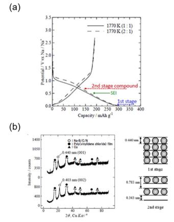
Fig. 15 Electrochemical insertion of Na $^+$  into B/C/N (Na-B/C/N). (a) Galvanostatic charge-discharge curves of B/C/N materials in 1 M NaPF $_6$  EC:DEC (1:1 v/v). (b) Ex situ XRD patterns of Na-B/C/N at 0.003 V and 0.70 V vs. Na $^+$ /Na, respectively. Modified with permission from ref. 97. Copyright 2015 Electrochemical Society of Japan.
