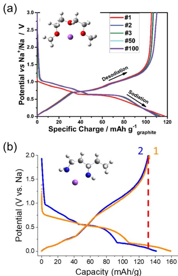
Fig. 16 Electrochemical cointercalation of  $\text{Na}^+$  in graphite. Charge/discharge curves of graphite in half-cells containing (a)  $\text{NaOTf}$  in diglyme and (b)  $\text{NaPF}_6$  in 1,3-diaminopentane. (a) was reproduced with permission from ref. 138. Copyright 2018 Wiley-VCH GmbH. (b) was reproduced with permission from ref. 141. Copyright 2024 The Authors.
