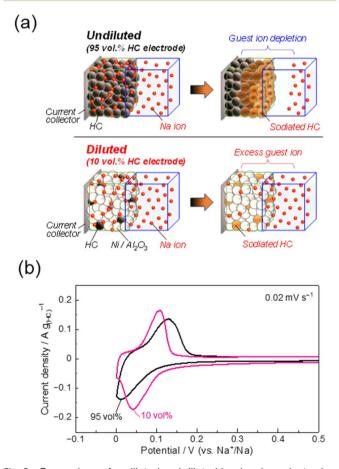
Fig. 8 Comparison of undiluted and diluted hard carbon electrodes. (a) Schematic of diluted electrodes method. (b) Cyclic voltammograms of sodium insertion/extraction of hard carbon obtained by using a three electrodes cell for diluted (10% AM) and conventional (95% AM) electrodes.
