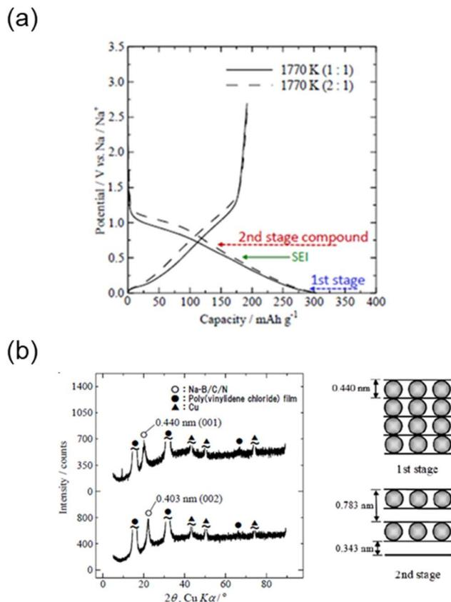
Fig. 15 Electrochemical insertion of  $\text{Na}^+$  into B/C/N (Na-B/C/N). (a) Galvanostatic charge–discharge curves of B/C/N materials in 1 M  $\text{NaPF}_6$  EC : DEC (1 : 1 v/v). (b) *Ex situ* XRD patterns of Na-B/C/N at 0.003 V and 0.70 V vs.  $\text{Na}^+/\text{Na}$ , respectively. Modified with permission from ref. 97. Copyright 2015 Electrochemical Society of Japan.
