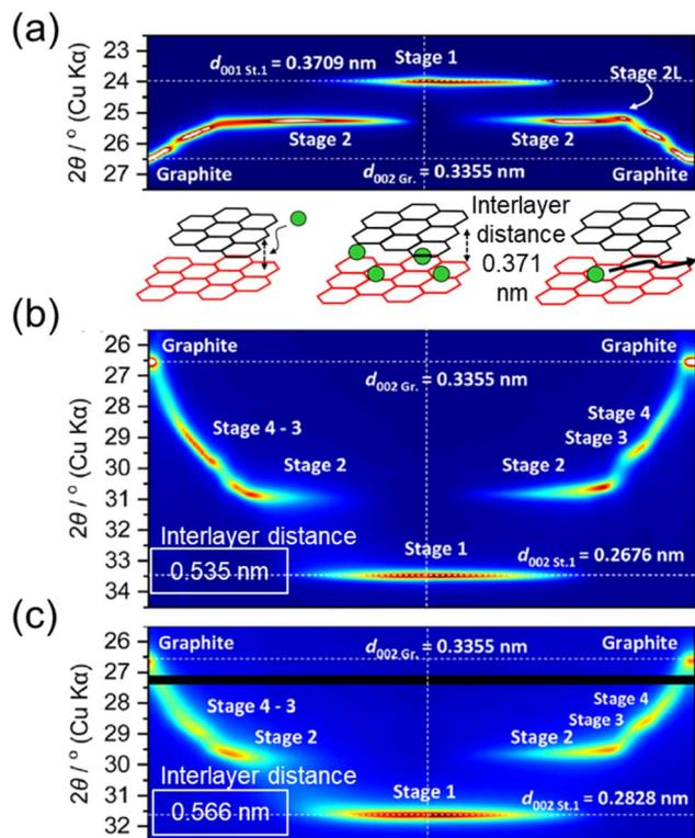
Fig. 12 *Operando* XRD of alkali intercalation at graphite in (a)  $\text{Li}^+$ , (b)  $\text{K}^+$  and (c)  $\text{Rb}^+$ -based ionic liquids. Below (a) is an illustration of the lattice space increase with ion insertion. All XRD data are modified with permission from ref. 86. Copyright 2023 Royal Society of Chemistry.
