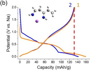
Fig. 16 Electrochemical cointercalation of Na $^+$  in graphite. Charge/ discharge curves of graphite in half-cells containing (a) NaOTf in diglyme and (b) NaPF $_6$  in 1,3-diaminopentane. (a) was reproduced with permission from ref. 138. Copyright 2018 Wiley-VCH GmbH. (b) was reproduced with permission from ref. 141. Copyright 2024 The Authors.
