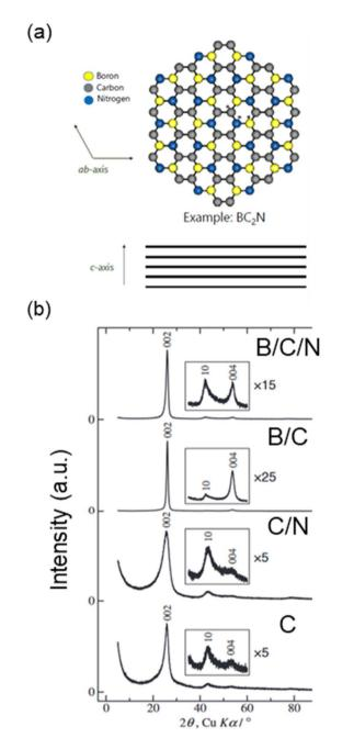
Fig. 14 Structure of B/C/N materials. (a) Graphite-like network of B/C/N (example:  $BC_2N$ ). (b) XRD patterns of B/C/N, B/C, C/N and C powders prepared using chemical vapor deposition. (b) is reproduced with permission from ref. 97. Copyright 2015 Electrochemical Society of Japan.
