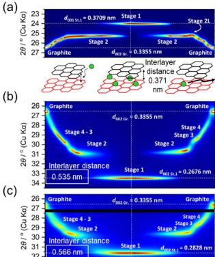
Fig. 12 Operando XRD of alkali intercalation at graphite in (a)  $Li^+$ , (b)  $K^+$  and (c)  $Rb^+$ -based ionic liquids. Below (a) is an illustration of the lattice space increase with ion insertion. All XRD data are modified with permission from ref. 86. Copyright 2023 Royal Society of Chemistry.
