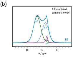
Fig. 17 Solvent dynamics during solvent cointercalation. (a) Illustration of  $\mathrm{Na}^+$  and diglyme interactions with graphite during cointercalation. (b) NMR response indicating the ratio of each solvent species. Reproduced with permission from ref. 154. Copyright 2022 Wiley-VCH GmbH.
