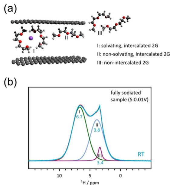
Fig. 17 Solvent dynamics during solvent cointercalation. (a) Illustration of Na<sup>+</sup> and diglyme interactions with graphite during cointercalation. (b) NMR response indicating the ratio of each solvent species. Reproduced with permission from ref. 154. Copyright 2022 Wiley-VCH GmbH.
