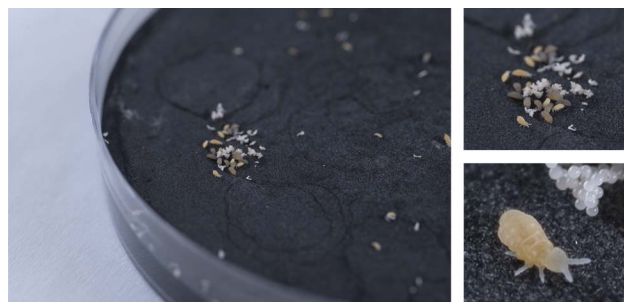
Fig. 2 Ceratophysella denticulata on a Petri dish ( \Phi 9.4 cm) filled with plaster of Paris and activated charcoal.
