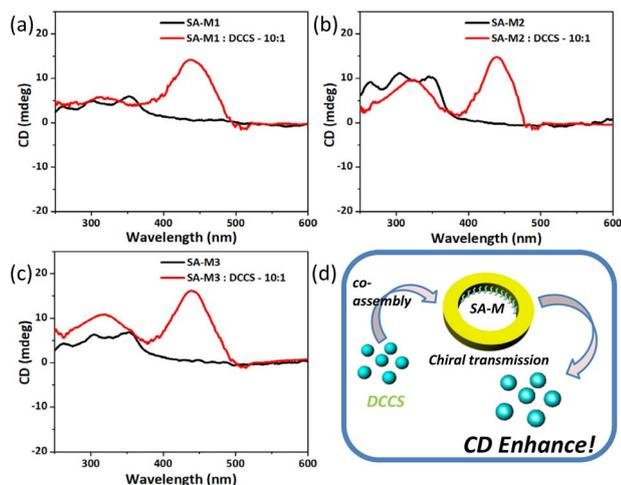
Fig. 5 (a–c) CD spectra of SA-M materials before and after co-assembly with DCCS in H<sub>2</sub>O/THF (v/v = 9/1). (d) Schematic representation of chiral transfer through co-assemblies.
