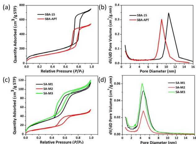
Fig. 2 (a) N<sub>2</sub> adsorption-desorption isotherms and (b) pore size distribution of SBA-15 and SBA-APT. (c) N<sub>2</sub> adsorption-desorption isotherms and (d) pore size distribution of SA-M materials.
