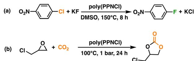
**Scheme 2** (a) Halogen-exchange reaction from CNB to FNB; (b) coupling reaction of CO<sub>2</sub> with GC.
