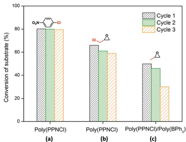
Fig. 3 Reaction conversions over three cycles (a) halogen-exchange, (b) CO<sub>2</sub>/GC coupling, and (c) CO<sub>2</sub>/PO coupling reactions. Conversion calculated by <sup>1</sup>H NMR spectroscopy. Conversions for recycled poly(PPNCl) were obtained from an average value of two trials.
