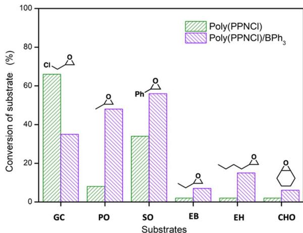
Fig. 2 CO<sub>2</sub>/epoxides coupling reaction to yield cyclic carbonates. Conversions calculated by <sup>1</sup>H NMR spectroscopy. Conversions for GC and PO were taken from the average value of three trials; the rest substrates were conducted once. Reactions were performed in a sealed ampoule on a 12.8 mmol scale at 0.1 mol% poly(PPNCl) with or without 0.1 mol% BPh<sub>3</sub> (0.1 mol% as calculated from the number of expected active functional groups).
