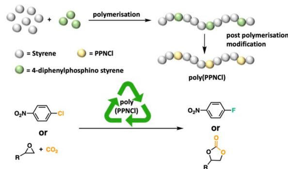
Fig. 1 (a) Previous work using PPNCl as catalysts; (b) poly(PPNCl) as a recyclable catalyst for halogen exchange and CO<sub>2</sub>/epoxide coupling reactions.
