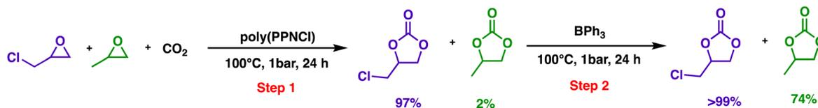
Scheme 3 The selective one-pot, two-step reaction of epoxide conversion to cyclic carbonates. General conditions: the feed ratio of GC : PO : poly(PPNCl) : BPh<sub>3</sub> is 1000 : 1000 : 4 : 4.
