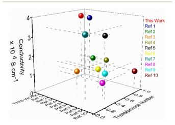
Fig. 5 Performance comparison plot of sodium ion conductivity (room temperature) and transference number of the nanosheets of AD-1 with the reported solid sodium ion conductor (refer to ESI, Table S4†).
