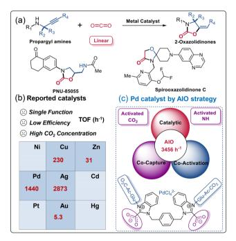
Fig. 1 (a) The metal-catalyzed cyclization of propargylic amines and  $CO_2$ . (b) The reported metal catalysts with different TOFs, see attached Table S1† for more detailed parameters. (c) Pd catalyst construct by integrated AIO strategy herein.
