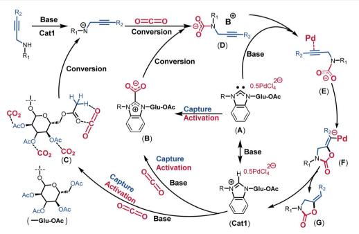
Proposed mechanism for Cat1-catalyzed carboxylative cyclization.
