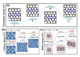
Fig. 5 (a) DFT optimized models for different S atom doping positions and formation energies of the four conformations. (b) Valence charge densities (the inset shows a 2D charge density image) and (c) Bader charges of the four nanozymes (the inset shows a differential charge density plot and red indicates charge accumulation, while blue indicates charge depletion).
