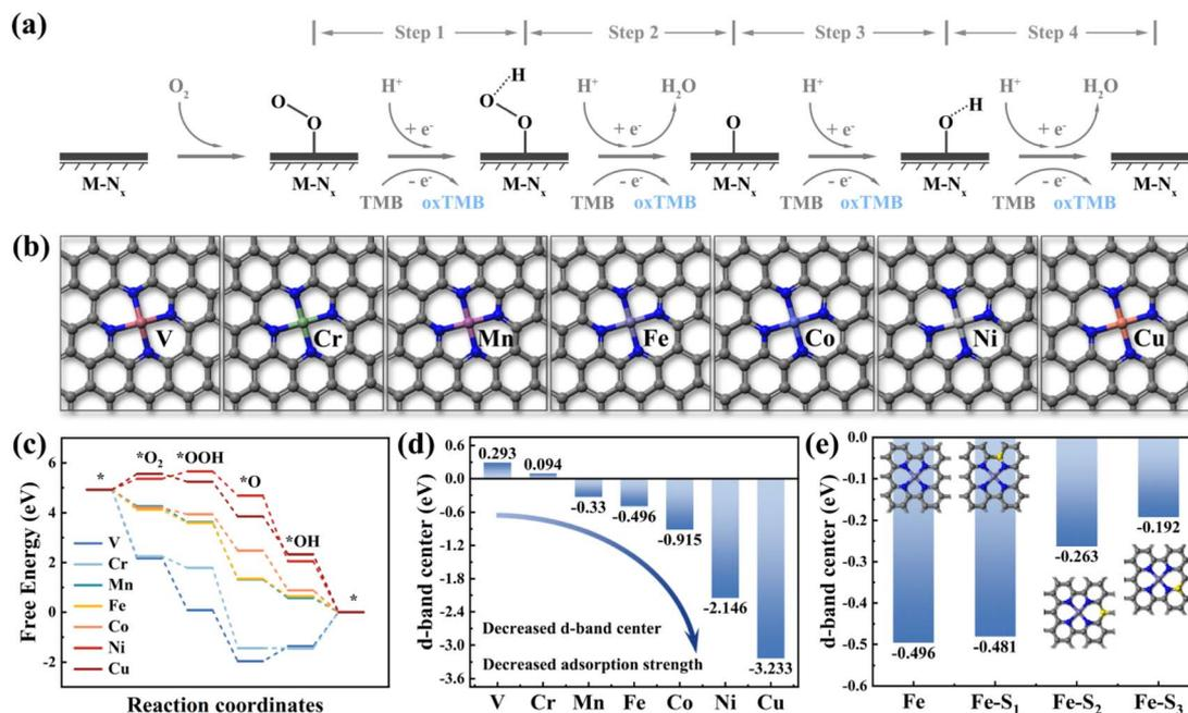
Fig. 1 (a) Schematic diagram of the catalytic reaction mechanism of oxidase-like activity at the  $M-N_4$  site. (b) Modeling of  $M-N_4$  ( $M = V, Cr, Mn, Fe, Co, Ni, Cu$ ) with different transition metals as central sites. (c) Step diagrams of adsorption energy changes and (d) d-band centers for seven  $M-N_4$  model oxidase-like catalytic reaction processes. (e) Histogram of d-band center changes for different S-doped sites.
