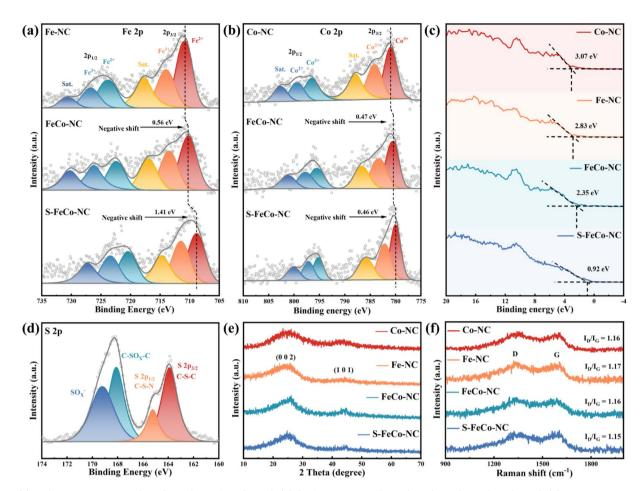
Fig. 3 (a) Fe 2p spectra of Fe-NC, FeCo-NC and S-FeCo-NC. (b) Co 2p spectra of Co-NC, FeCo-NC and S-FeCo-NC. (c) Valence band spectra of all samples. (d) S 2p spectra of S-FeCo-NC. Superimposed (e) XRD and (f) Raman spectral profiles of four nanozymes.
