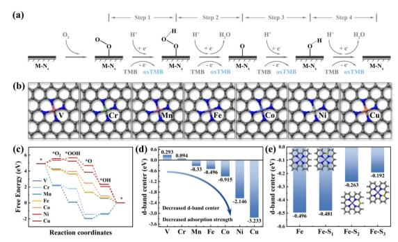
Fig. 1 (a) Schematic diagram of the catalytic reaction mechanism of oxidase-like activity at the  $M-N_X$  site. (b) Modeling of  $M-N_4$  (M=V, Cr, Mn, Fe, Co, Ni, Cu) with different transition metals as central sites. (c) Step diagrams of adsorption energy changes and (d) d-band centers for seven  $M-N_4$  model oxidase-like catalytic reaction processes. (e) Histogram of d-band center changes for different S-doped sites.
