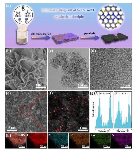
Fig. 2 (a) Schematic diagram of the S-FeCo-NC synthesis process. (b) SEM, (c) TEM, and (d) HRTEM images. (e and f) AC-HAADF-STEM characterization images and Fe/Co dual-atom pairs are marked using red boxes. (g) Intensity distribution of dual-atom sites. (h) EDS mapping of S-FeCo-NC.
