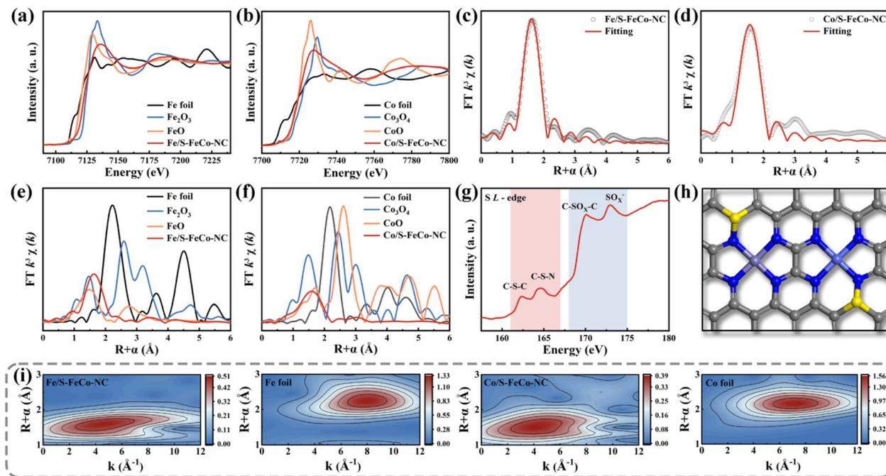
Fig. 4 XANES spectrum of the (a) Fe and (b) Co K-edge. EXAFS of (c) Fe and (d) Co sites in S-FeCo-NC in  $R$ -space and the corresponding fitted curves. Comparative plots of (e) Fe and (f) Co sites with control samples in  $R$ -space. XANES spectrum of the (g) S L-edge. (h) The most probable atomic configuration of S-FeCo-NC. Color scheme: gray for C, dark blue for N, yellow for S, purple for Fe, and light blue for Co. (i) WT spectra of Fe, Co and control samples in S-FeCo-NC.
