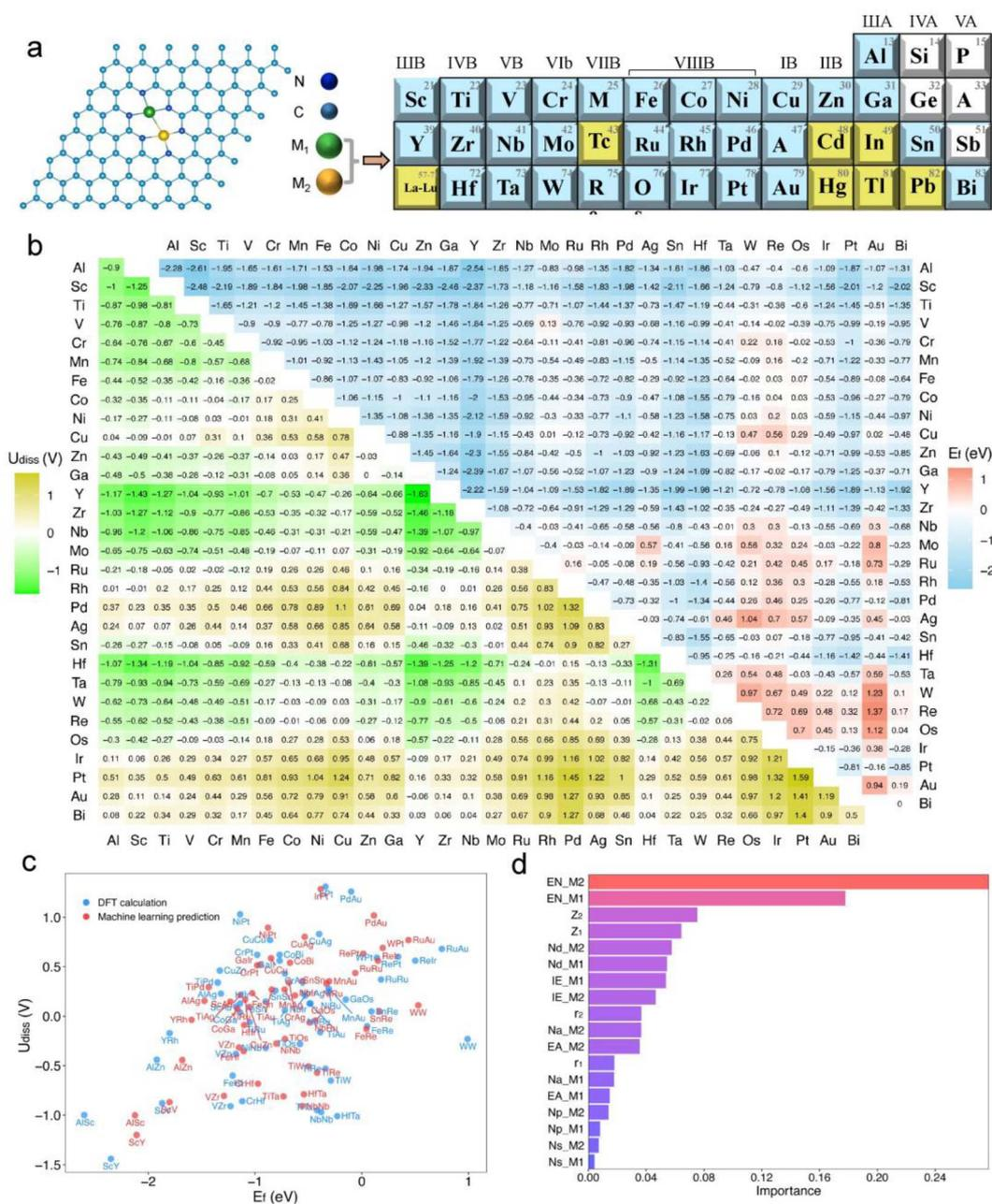
Fig. 2 (a) Structure of the graphene-based bimetallic catalyst (M1M2-N6@Gra). (b) Calculated formation energy ( $E_f$ , in eV) and dissolution potential ( $U_{diss}$ , in V) of metal atoms in M1M2-N6@Gra. (c) Machine learning predictions of  $U_{diss}$  and  $E_f$  compared with DFT calculations. (d) Feature importance analysis based on a random forest model algorithm in machine learning.
