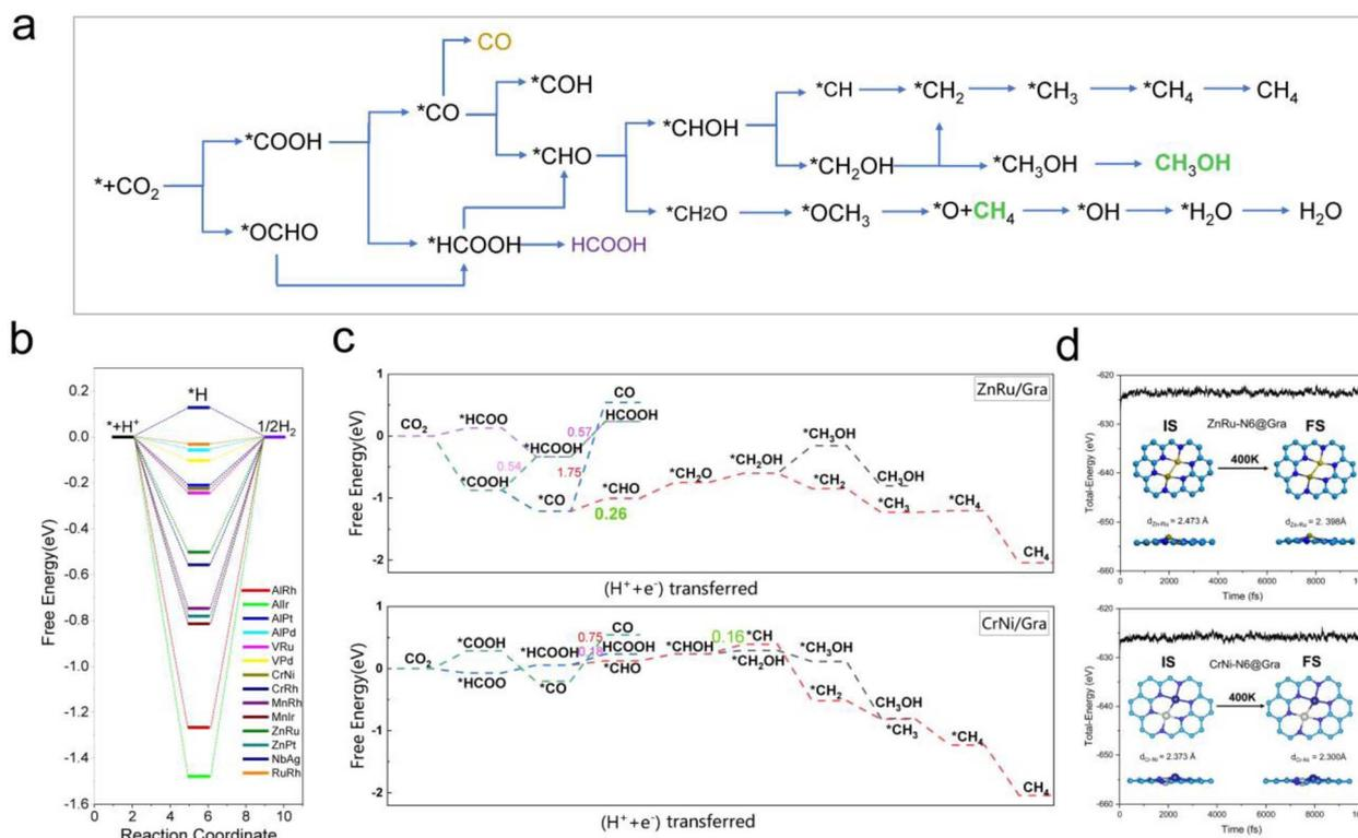
Fig. 7 (a) Possible reaction pathways of the  $CO_2RR$  on M1M2-N6@Gra catalysts. (b) Free energy graphs of HER side reactions on 14 M1M2-N6@Gra catalysts. (c) The free energy diagrams of ZnRu-N6@Gra and CrNi-N6@Gra in reducing  $CO_2$  to  $CH_4$  and  $CH_3OH$  pathways highlight the rate limiting steps of methane production with green bold numbers. (d) Fluctuations of energy at 400 K for catalysts ZnRu-N6@Gra and CrNi-N6@Gra with atomic structure snapshots shown in insets.
