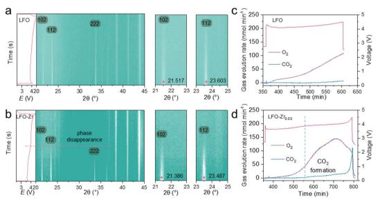
Fig. 6 Phase conversion and evolution of oxygen in the initial charge of LFO and LFO- $Zr_{0.03}$ . The corresponding 2D contour plot and magnified details of the (102) and (112) peaks of LFO (a) and LFO- $Zr_{0.03}$  (b), and quantitative DEMS data for  $O_2$  and  $CO_2$  released in the LFO (c) and LFO- $Zr_{0.03}$  (d) during the first charge to 4.5 V.
