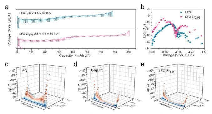
Fig. 4 Kinetic properties of LFO and LFO- $Zr_{0.03}$  electrodes. (a) Galvanostatic intermittent titration technique (GITT) profiles and (b) the  $log(D_{Li^+})$ -potential plots during charge processes. The *in situ* EIS of LFO (c), C@LFO (d) and LFO- $Zr_{0.03}$  (e) during the initial de-lithiation process.
