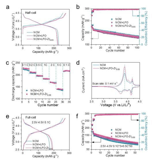
Electrochemical performances of half-cell and full-cell electrodes of NCM, NCM with LFO and LFO-Zr<sub>0.03</sub>. (a) The initial charge/discharge curves. (b) Cycle performance. (c) Rate performances. (d) CV curves at  $0.1 \, \text{mV} \, \text{s}^{-1}$  scan rates. (e) The initial charge/discharge curve and (f) cycle performance of the full-cell
