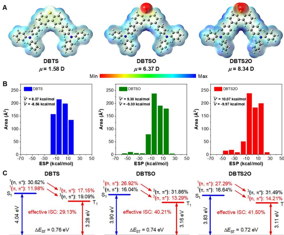
Fig. 3 The theoretical calculation results of DBTS, DBTSO, and DBTS2O. (A) ESP distributions and dipole moment ( $\mu$ ). (B) The histograms of electrostatic potential area distribution, positive average ESP value ( $\bar{V}^+$ ) and negative average ESP value ( $\bar{V}^-$ ). (C) Calculated energy levels of  $S_1$  and  $T_1$  states, and the proportions of  $^1(n, \pi^*)$ ,  $^3(n, \pi^*)$ ,  $^1(\pi, \pi^*)$  and  $^3(\pi, \pi^*)$ .
