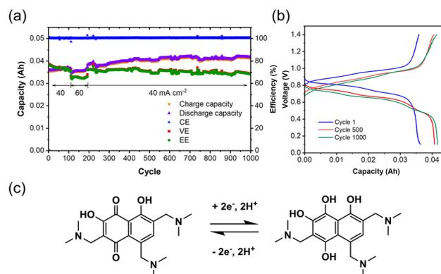
Fig. 4 Battery performance of TANQ after electrosynthesis: (a) cycling performance, (b) charge and discharge profiles, (c) structural change of TANQ during charge-discharge cycling. The flow cell was 0.1 M TAND/0.5 M  $\text{V}^{2+}$  in 3 M  $\text{H}_2\text{SO}_4$  cycled at 40  $\text{mA cm}^{-2}$  (cycle 111–192 temporarily operated at 60  $\text{mA cm}^{-2}$ ).
