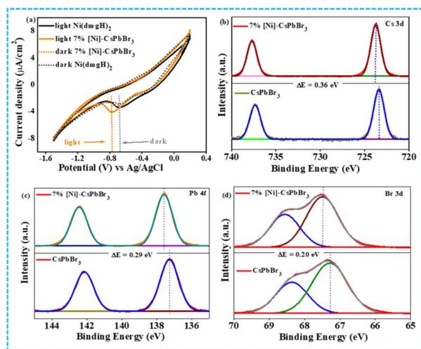
**Fig. 2** (a) Cyclic voltammogram of CsPbBr<sub>3</sub> QDs and 7% [Ni]-CsPbBr<sub>3</sub> in the dark and light. XPS spectra of CsPbBr<sub>3</sub> and 7% [Ni]-CsPbBr<sub>3</sub> (b) Cs 3d, (c) Pb 4f, (d) Br 3d.
