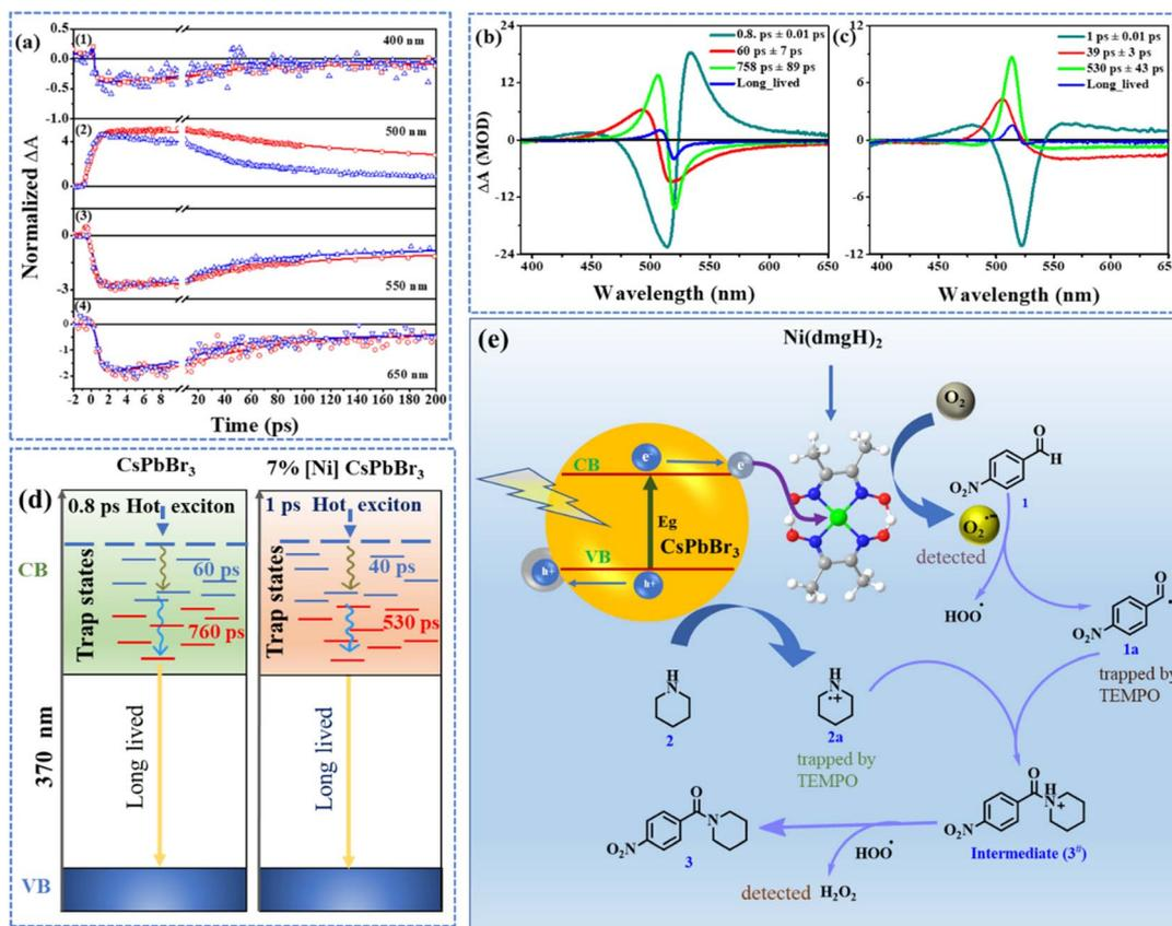
Fig. 3 (a) Kinetic traces at (1) 400 nm (2) 500 nm (3) 550 nm and (4) 650 nm for CsPbBr<sub>3</sub> (red) and 7% [Ni]-CsPbBr<sub>3</sub> (blue). The solid lines are fitted lines. The decay-associated spectra (DAS) of (b) CsPbBr<sub>3</sub> and (c) 7% [Ni]-CsPbBr<sub>3</sub>. (d) Schematic illustration of the formation and relaxation of charge carriers of CsPbBr<sub>3</sub> and 7% [Ni]-CsPbBr<sub>3</sub>. (e) Proposed mechanism of C–N bond formation.
