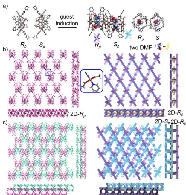
Fig. 7 (a) The transformation of **P6PhPy4** (*R*<sub>p</sub>, *S*<sub>p</sub>) in **sbl-2D-P6MOCN**. (b) The crystal structure and diagram of a sandwich bilayer 2D coordination of the polymer **sbl-2D-P6MOCN** (2D-*R*<sub>p</sub>). (c) The stacking diagram of a sandwich bilayer 2D coordination of the polymer **sbl-2D-P6MOCN** (2D-*R*<sub>p</sub> and 2D-*S*<sub>p</sub>). Noncoordinated solvent molecules were omitted.
