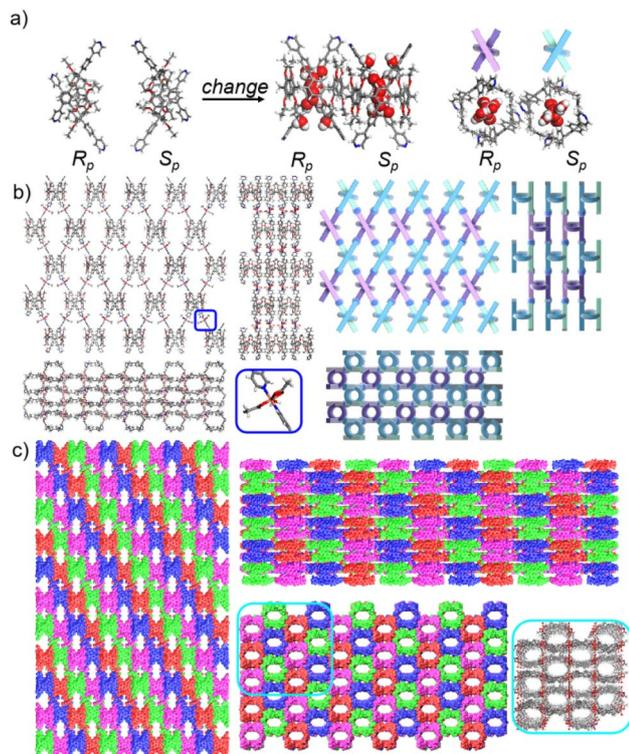
Fig. 4 (a) The crystal structure and diagram of **P6PhPy4** ( $R_p$ ,  $S_p$ ) in **mtl-2D-P6MOCN**. (b) The crystal structure and diagram of a multi-layer 2D coordination of the polymer **mtl-2D-P6MOCN**. (c) The stacking structure of a multi-layer 2D coordination of the polymer **mtl-2D-P6MOCN**. Noncoordinated solvent molecules were omitted.
