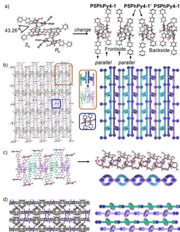
Fig. 2 (a) The transformation of **P5PhPy4** ( $R_p$ ,  $S_p$ ) in **ml-2D-P5MOCN**. (b) The top view of a single layer 2D coordination of the polymer **ml-2D-P5MOCN**. (c) The side view of the alternate  $-R_p-S_p-R_p-S_p-$  arrangement of the polymer **ml-2D-P5MOCN**. (d) The stacking structure of **ml-2D-P5MOCN**. Noncoordinated solvent molecules are omitted.
