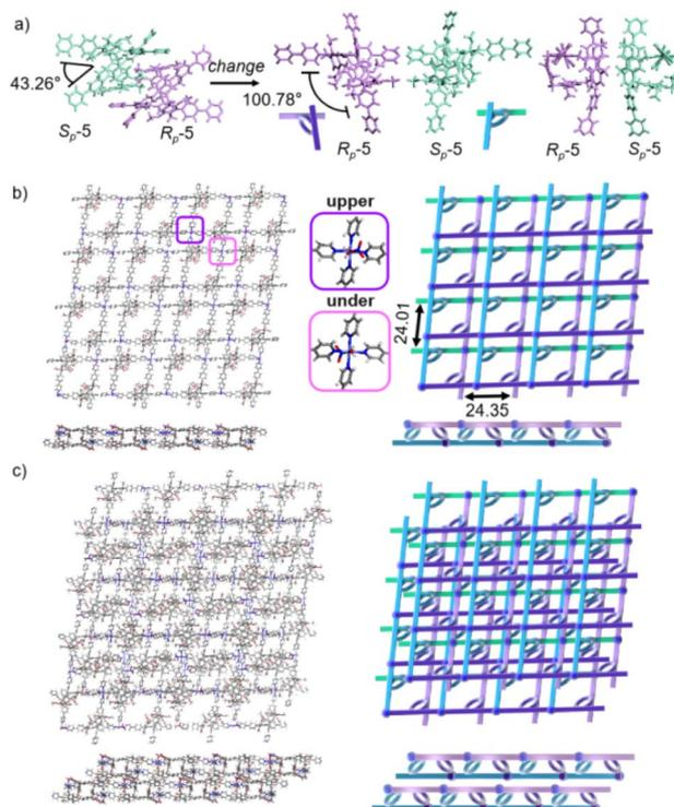
Fig. 3 (a) The transformation of **P5PhPy4** ( $R_p$ ,  $S_p$ ) in **bl-2D-P5MOCN**. (b) The crystal structure and diagram of a bilayer 2D coordination of the polymer **bl-2D-P5MOCN**. (c) The stacking structure of a bilayer 2D coordination of the polymer **bl-2D-P5MOCN**. Noncoordinated solvent molecules are omitted.
