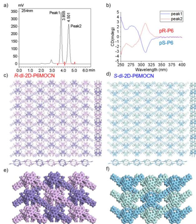
Fig. 8 (a) Resolution of the enantiomers of P6PhPy4 by chiral HPLC. (b) CD spectra of *S*-P6PhPy4 (blue line) and *R*-P6PhPy4 (red line) in dichloromethane. (c and d) The crystal structure bilayer 2D coordination of the polymers *R*-bl-2D-P6MOCN and *S*-bl-2D-P6MOCN. (e and f) The up and down entanglement pattern of *R*-bl-2D-P6MOCN and *S*-bl-2D-P6MOCN. Noncoordinated solvent molecules were omitted.
