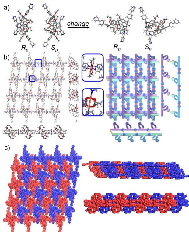
Fig. 6 (a) The crystal structure and diagram of **P6PhPy4** ( $R_p$ ,  $S_p$ ) in **fl-2D-P6MOCN**. (b) The crystal structure and diagram of a four-layer 2D coordination of the polymer **fl-2D-P6MOCN**. (c) The four-layer braided two-dimensional network of **fl-2D-P6MOCN** with the up and down entanglement pattern and interlocking pattern. Noncoordinated solvent molecules were omitted.
