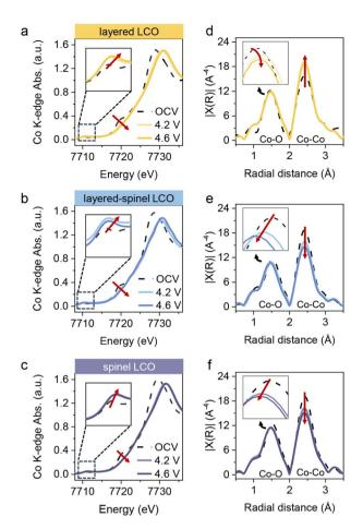
Fig. 4 (a-c) Normalized ex situ Co K-edge XANES spectra at states of pristine, 4.2 V and 4.6 V (vs. Li/Li<sup>+</sup>) for (a) layered LCO, (b) layeredspinel LCO and (c) spinel LCO. (d-f) Co K-edge EXAFS spectra at states of pristine, 4.2 V and 4.6 V (vs. Li/Li+) for (d) layered LCO, (e) layeredspinel LCO and (f) spinel LCO
