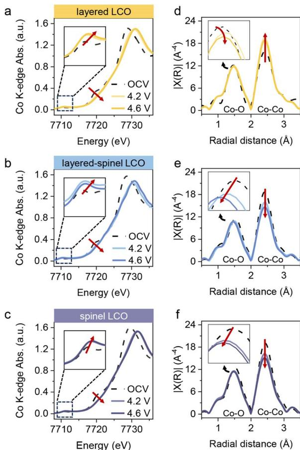
Fig. 4 (a–c) Normalized *ex situ* Co K-edge XANES spectra at states of pristine, 4.2 V and 4.6 V (vs. Li/Li<sup>+</sup>) for (a) layered LCO, (b) layered-spinel LCO and (c) spinel LCO. (d–f) Co K-edge EXAFS spectra at states of pristine, 4.2 V and 4.6 V (vs. Li/Li<sup>+</sup>) for (d) layered LCO, (e) layered-spinel LCO and (f) spinel LCO.
