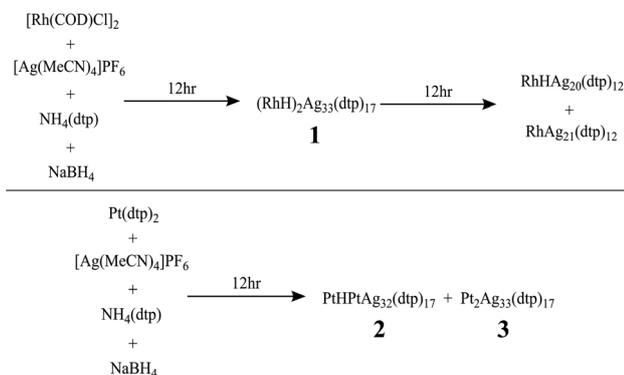
Fig. 2 Synthesis and decomposition of the hydride-containing supermolecules.
