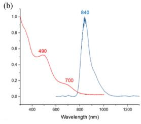
Fig. 6 Absorption (2-MeTHF, RT, red) and emission (2-MeTHF glass, 77 K, blue) spectra of (a) 1 (b) 2.
