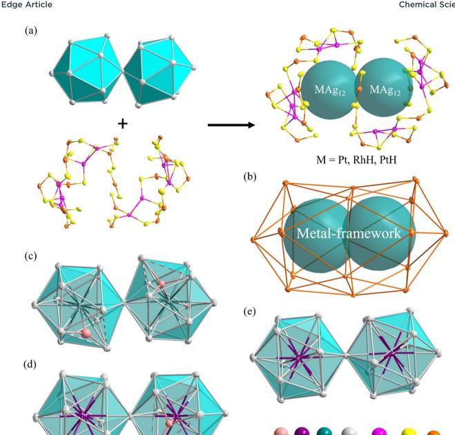
Fig. 4 (a) The disassembly diagram of a superatomic molecule and passivating layer. (b) Interpenetrated icosahedra composed of 17 P atoms (c) the (RhH)<sub>2</sub>Ag<sub>23</sub> bi-icosahedral core of 1 (d) the (PtH)PtAg<sub>23</sub> bi-icosahedral core of 2 (e) the Pt<sub>2</sub>Ag<sub>23</sub> bi-icosahedral core of 3.
