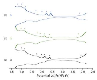
Fig. 7 DPV curves of (a) 1 (b) 2 (c) 3 were obtained in a 0.1 M DCM solution of  $Bu_4NPF_6$  at 233 K. (Potential increments: 2 mV; pulse amplitude: 50 mV; pulse width: 50 ms; sampling width: 25 ms; pulse period: 100 ms.).
