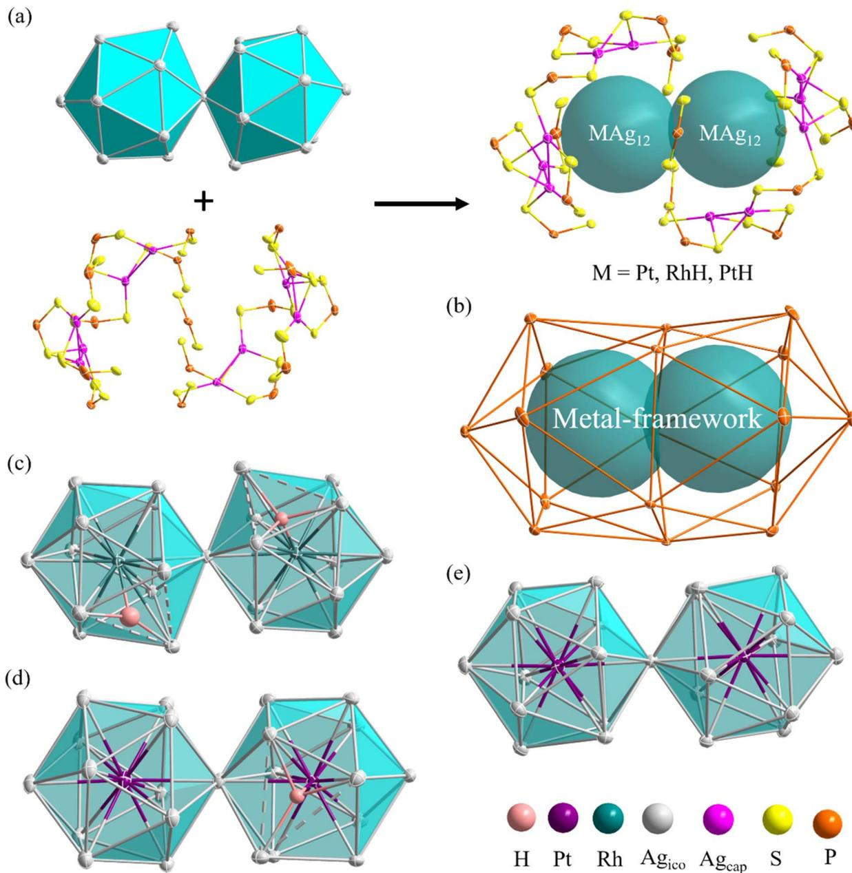
Fig. 4 (a) The disassembly diagram of a superatomic molecule and passivating layer. (b) Interpenetrated icosahedra composed of 17 P atoms (c) the  $(RhH)_2Ag_{23}$  bi-icosahedral core of 1 (d) the  $(PtH)PtAg_{23}$  bi-icosahedral core of 2 (e) the  $Pt_2Ag_{23}$  bi-icosahedral core of 3.
