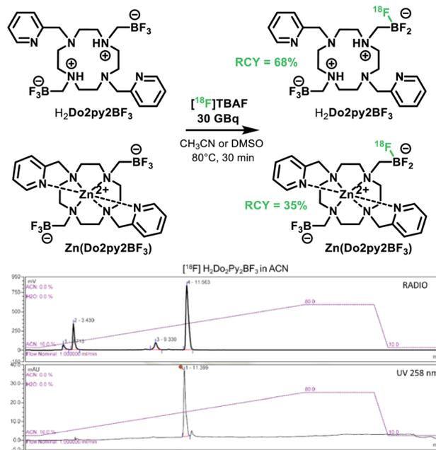
Scheme 4 <sup>18</sup>F-radiolabeling of H<sub>2</sub>Do2py2BF<sub>3</sub> and Zn(Do2py2BF<sub>3</sub>) in acetonitrile, and corresponding HPLC (UV) and radioHPLC traces for H<sub>2</sub>Do2py2BF<sub>3</sub>.
