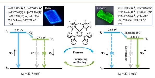
Fig. 1 The PL image and crystal unit cell parameters of B-form and G-form crystals. The molecular structure of ArBFO. Proposed energy level structure of B-form and G-form aggregates during the pressure-fumigating or pressure-heating process.
