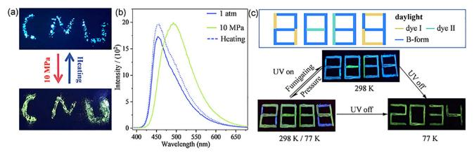
Fig. 5 (a and b) Photos (a) and PL spectra (b) of the B-form powder during the pressure—heating process. (c) Information encryption photos made with dye I, dye II, and the B-form powder of ArBFO. The UV light illumination is 365 nm.
