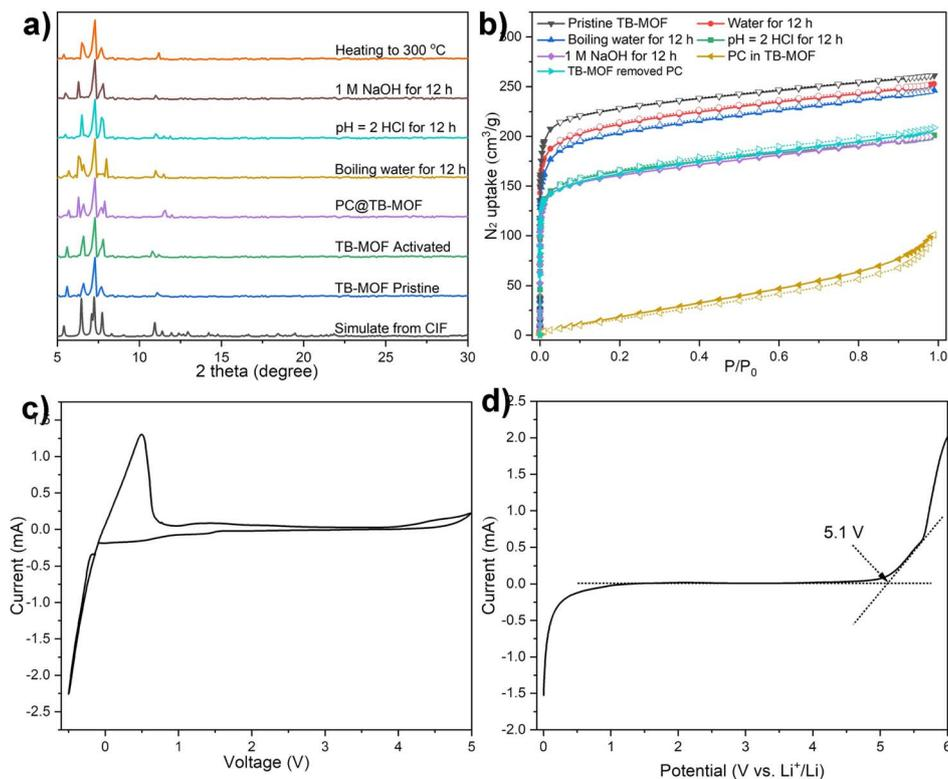
Fig. 2 (a) PXRD patterns of TB-MOF under different conditions. (b) The corresponding N<sub>2</sub> adsorption isotherms at 77 K. (c) CV and (d) LSV measurements for the SS/TB-MOF/Li asymmetric cells at room temperature at a scan speed of 5 mV s<sup>-1</sup>.
