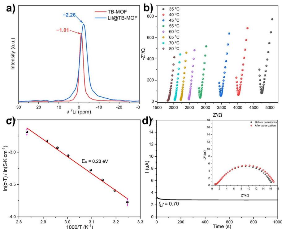
Fig. 3 (a)  $^7\text{Li}$  MAS NMR spectra of TB-MOF and LiI@TB-MOF. (b) Nyquist plots for TB-MOF. (c) Ionic conductivity as a function of temperature. (d) Current–time curve for the LiI/TB-MOF/LiI cell at a DC polarization of 10 mV. Inset: Nyquist plots obtained before and after polarization.
