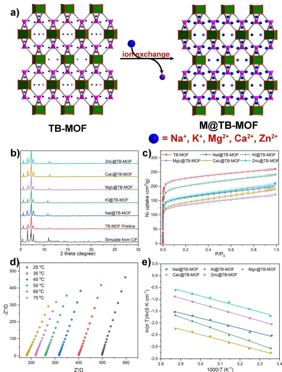
Fig. 5 (a) Schematic illustration of the grafting of other metal iodides into TB-MOF. (b) PXRD and (c) N<sub>2</sub> adsorption isotherms of the resulting M<sub>x</sub>@TB-MOF. (d) Nyquist plots of MgI<sub>2</sub>@TB-MOF. (e) Arrhenius plots for the ionic conductivity of NaI@TB-MOF, KI@TB-MOF, MgI<sub>2</sub>@TB-MOF, CaI<sub>2</sub>@TB-MOF, and ZnI<sub>2</sub>@TB-MOF.
