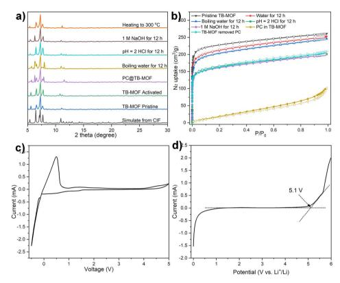
Fig. 2 (a) PXRD patterns of TB-MOF under different conditions. (b) The corresponding  $N_2$  adsorption isotherms at 77 K. (c) CV and (d) LSV measurements for the SS/TB-MOF/Li asymmetric cells at room temperature at a scan speed of 5 mV s<sup>-1</sup>.
