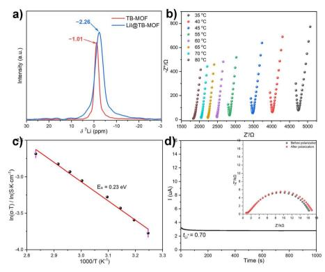
Fig. 3 (a) <sup>7</sup>Li MAS NMR spectra of TB-MOF and Lil@TB-MOF. (b) Nyquist plots for TB-MOF. (c) Ionic conductivity as a function of temperature. (d) Current-time curve for the Li/TB-MOF/Li cell at a DC polarization of 10 mV. Inset: Nyquist plots obtained before and after polarization.
