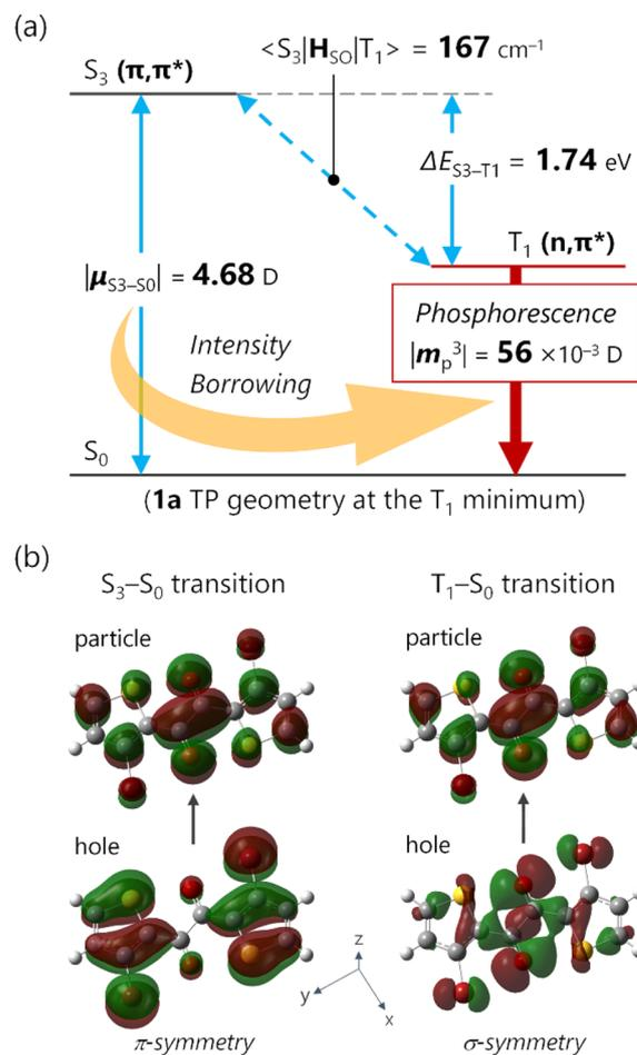
Fig. 5 (a) Energy diagram of **1a** in the  $T_1$ -optimized *trans*-planar (TP) geometry depicting the principal intensity-borrowing. Energies, the transition dipole moment  $\mu_{S_3-S_0}$ , and the spin-orbit coupling matrix element  $\langle S_3 | \mathbf{H}_{SO} | T_1 \rangle$  were calculated at the TDA/(u)CAM-B3LYP-D3/6-311G(d) level. (b) Principal natural transition orbitals (NTOs) for  $S_3$ - $S_0$  (left) and  $T_1$ - $S_0$  (right) transitions.
