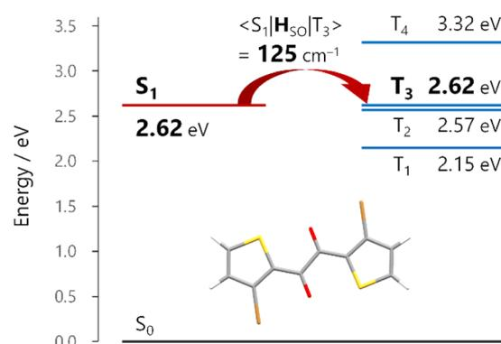
Fig. 4 Energy diagram of **1a** in the S<sub>1</sub>-optimized *trans*-planar (TP) geometry. Energies and the spin-orbit coupling matrix element between the S<sub>1</sub> and T<sub>3</sub> states ( $\langle S_1 | \mathbf{H}_{SO} | T_3 \rangle$ ) were calculated at the TDA/uCAM-B3LYP-D3/6-311G(d) level of theory.
