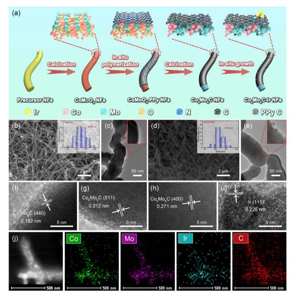
Fig. 1 (a) Synthetic scheme of  $Co_6Mo_6C$ -Ir-2 NFs. (b and d) SEM and (c and e) TEM images of  $Co_6Mo_6C$  NFs and  $Co_6Mo_6C$ -Ir-2 NFs. Insets of (b and d): diameter distributions of  $Co_6Mo_6C$  NFs and  $Co_6Mo_6C$ -Ir-2 NFs. (f-i) HRTEM images and (j) HAADF-STEM image and corresponding elemental mapping images of  $Co_6Mo_6C$ -Ir-2 NFs.
