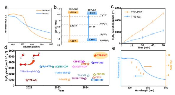
Fig. 2 (a) UV/vis DRS spectra and (b) band structures of TPE-PNZ and TPE-AC. (c) Typical time course of  $H_2O_2$  production in pure water using TPE-PNZ and TPE-AC, error bars are derived from standard errors from three tests. (d) Summary of  $H_2O_2$  production rates from recently reported CMP-based photocatalysts for  $H_2O_2$  production. (e) Wavelength-dependent AQEs of TPE-PNZ, error bars are derived from standard errors from three tests.
