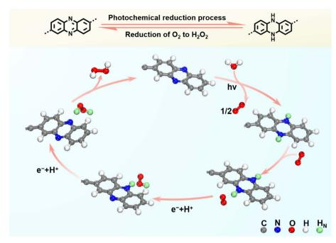
Fig. 5 Schematic illustration of the reversible transformation between phenazine and dihydrophenazine in TPE-PNZ during  $H_2O_2$  production. (Color denotation: gray: C; blue: N; red: O; white: H in benzene; green: H in dihydrophenazine).
