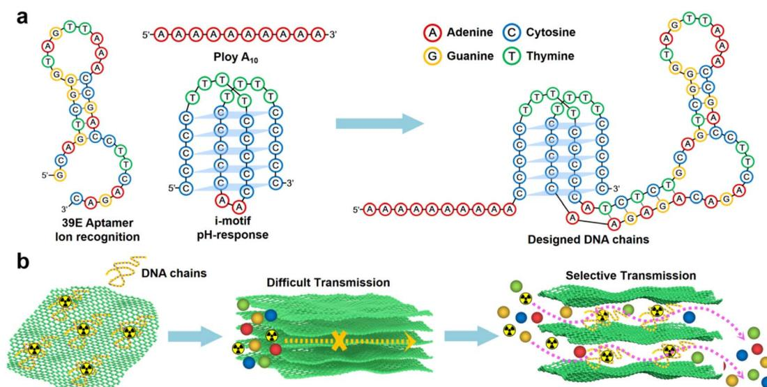
**Scheme 1** Schematic illustration of a 2D membrane with ion recognition channels. (a) Schematic representation of DNA fragments composed of poly  $A_{(10)}$ , U Aptamer and i-motif fragments. (b) Construction strategy of the 2D separation membrane.
