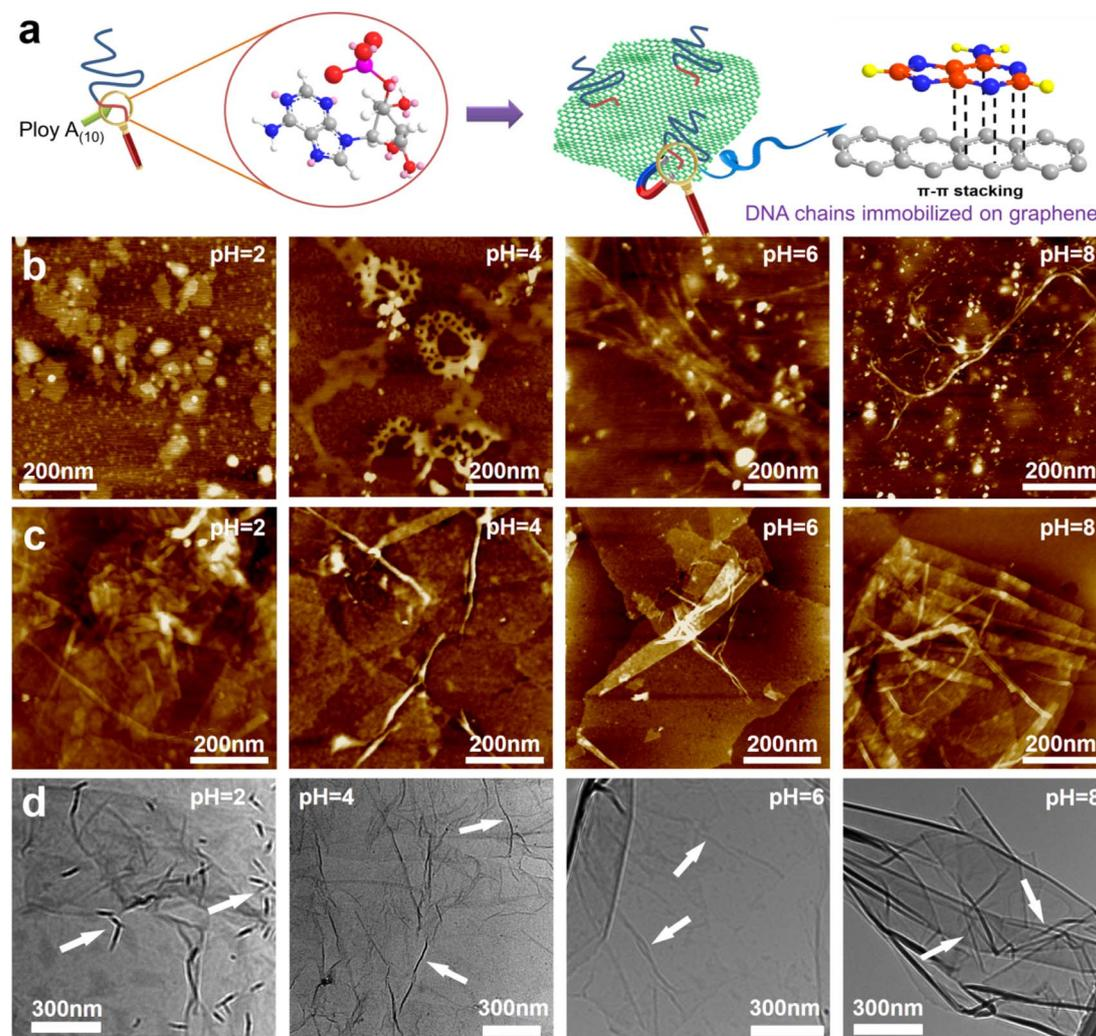
Fig. 1 Interaction between GO and DNA. (a) Schematic diagram of  $\pi$ – $\pi$  stacking between DNA bases and GO. (b) AFM images of DNA at pH = 2, 4, 6 and 8. The white particles in the image are crystals of the buffer solution used to adjust the pH. AFM image (c) and TEM image (d) of the mixture of GO and DNA at pH = 2, 4, 6 and 8.
