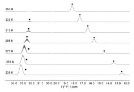
Fig. 2 <sup>31</sup>P NMR spectra of a sample of a mixture of 1 and CS<sub>2</sub> at different temperatures. The peaks of the FLP 1 (●) and of the CS<sub>2</sub> adduct 2 ( ) are labelled.
